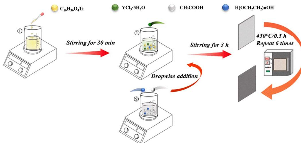
Fig. 1 The preparation process of the Ti/TiO<sub>2</sub> cathode.
