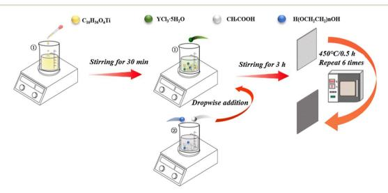
Fig. 1 The preparation process of the Ti/TiO<sub>2</sub> cathode.
