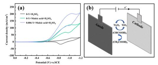
Fig. 9 (a) CV curve of the 0-Y electrode in  $1 \text{ M H}_2\text{SO}_4$  and 1 M maleic acid  $+ 0.5 \text{ M H}_2\text{SO}_4$  solution and the CV curve of the 0.006-Y electrode in 1 M maleic acid  $+ 0.5 \text{ M H}_2\text{SO}_4$  solution. (b) Indirect reduction of maleic acid to succinic acid on a Ti/TiO<sub>2</sub> film electrode.
