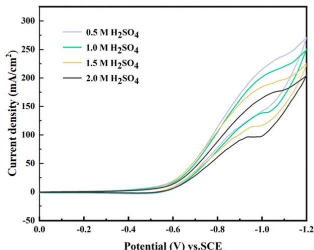
Fig. 12 CV curves of maleic acid at the 0.006-Y electrode with different electrolyte concentrations.
