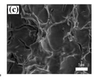
Fig. 14 (a) FT-IR spectrum of maleic acid. (b) FT-IR spectrum of succinic acid products. (c) SEM image of the electrode after continuous electrolysis for 24 hours.
