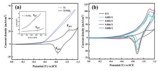
Fig. 7 (a) CV curves of the Ti and Ti/TiO<sub>2</sub> electrodes at 1 M H<sub>2</sub>SO<sub>4</sub>. (b) CV curves of different electrodes at 1 M H<sub>2</sub>SO<sub>4</sub>.
