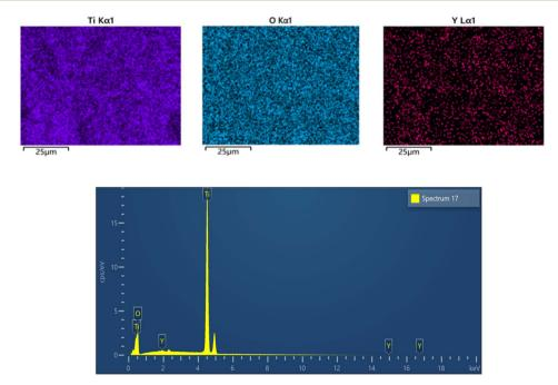
Fig. 5 EDS of the 0.006-Y electrodes.
