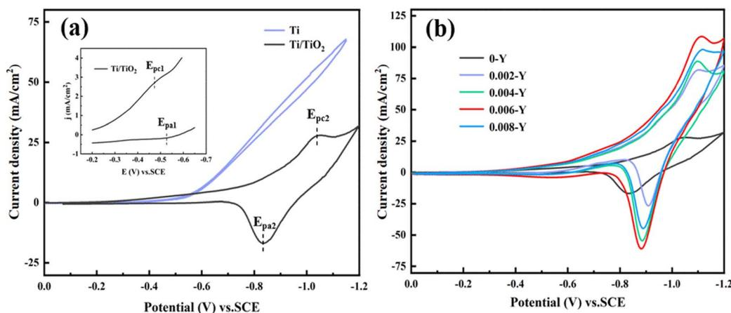
Fig. 7 (a) CV curves of the Ti and Ti/TiO<sub>2</sub> electrodes at 1 M H<sub>2</sub>SO<sub>4</sub>. (b) CV curves of different electrodes at 1 M H<sub>2</sub>SO<sub>4</sub>.
