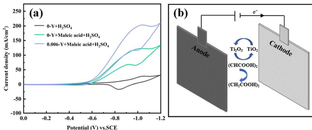
Fig. 9 (a) CV curve of the 0-Y electrode in 1 M H<sub>2</sub>SO<sub>4</sub> and 1 M maleic acid + 0.5 M H<sub>2</sub>SO<sub>4</sub> solution and the CV curve of the 0.006-Y electrode in 1 M maleic acid + 0.5 M H<sub>2</sub>SO<sub>4</sub> solution. (b) Indirect reduction of maleic acid to succinic acid on a Ti/TiO<sub>2</sub> film electrode.
