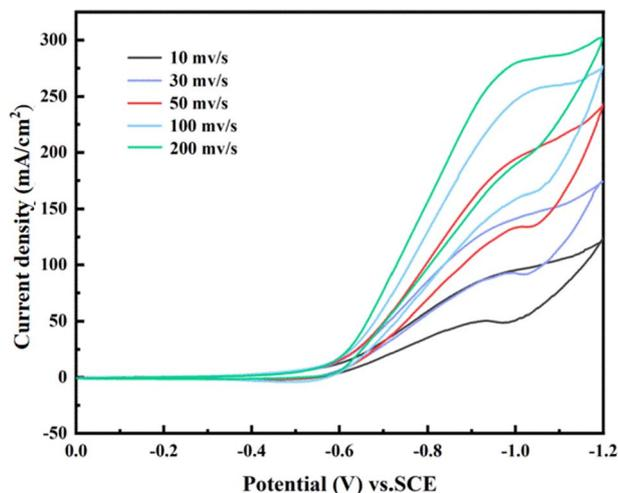
Fig. 10 CV curves of maleic acid at different sweep speeds at 0.006-Y electrodes.
