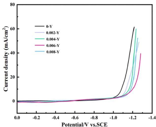
Fig. 6 LSV curves of different electrodes at 1 M H<sub>2</sub>SO<sub>4</sub>.
