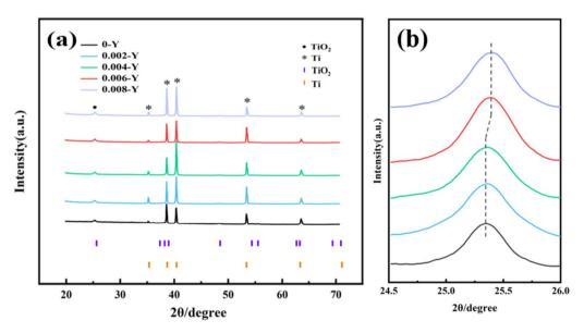
Fig. 3 (a) XRD patterns of different electrodes and (b) partially enlarged XRD patterns.
