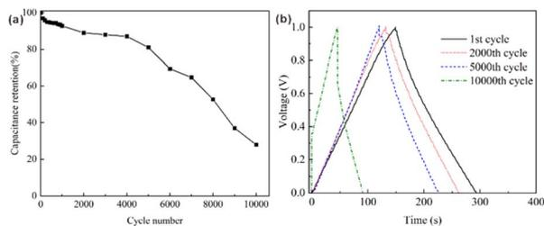
Fig. 2 (a) The capacitance retention of the symmetric supercapacitor over 10 000 cycles at  $1 \text{ A g}^{-1}$  and (b) GCD curves of the symmetric supercapacitor at different numbers of cycles at  $1 \text{ A g}^{-1}$ .
