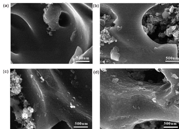
Fig. 8 SEM images of RHC in the positive electrode of SCs with varying  $m_+/m_-$  ratios at 2 (a), 1.5 (b), 1.25 (c), 1 (d) after 10 000 GCD cycles.
