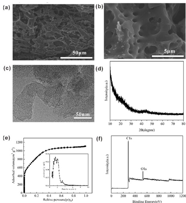
Fig. 1 (a) Low-magnification SEM image; (b) high-magnification SEM image; (c) TEM image; (d) X-ray diffraction pattern; (e)  $N_2$  adsorption–desorption isotherms (inset is the corresponding pore size distribution); and (f) XPS survey scan of RHC.
