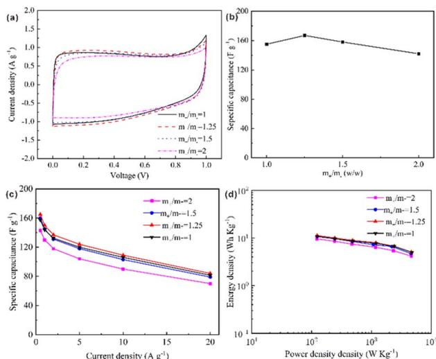
Fig. 6 (a) CV curves of SCs with varying  $m_+/m_-$  ratios at a scan rate of  $5 \text{ mV s}^{-1}$ ; (b) specific capacitance of SCs with varying  $m_+/m_-$  ratios at a scan rate of  $5 \text{ mV s}^{-1}$ ; (c) specific capacitance of SCs with varying  $m_+/m_-$  ratios at the different current density; (d) Ragone plots of SCs with varying  $m_+/m_-$  ratios.
