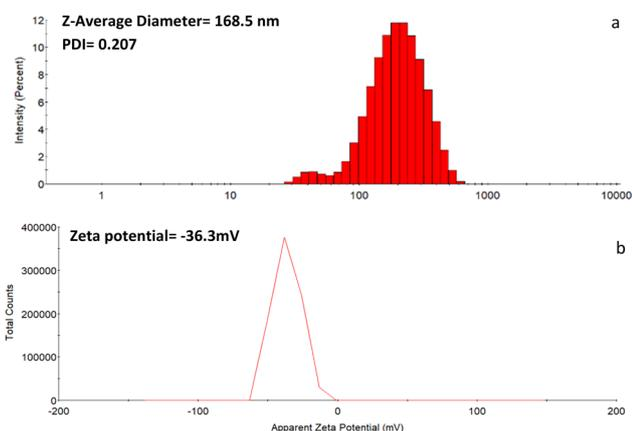
Fig. 3 Spectra of (a) particle size distribution, PDI, and (b) zeta potential of phytofabricated silver nanoparticles (MdSE-Ag/AgCl-NPs).
