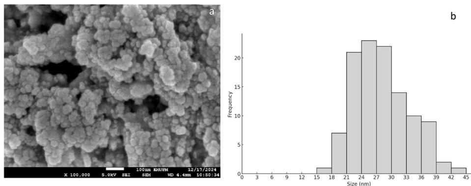
Fig. 5 (a) Field emission scanning electron microscopy (FESEM) image detailing surface morphology of the synthesized MdSE-Ag/AgCl nanoparticles and (b) histogram showing size distributions of the nanoparticles.
