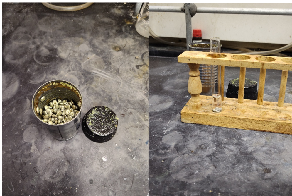
Fig. 1 Tomato paste milling jar after grinding a reaction with eugenol as a nucleophile (left) and solvent extraction of beads with chloroform for analysis of the ether product 28 (right).
