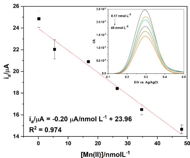
Fig. 7 Linear range of the anodic ( $i_a$ ) peak currents of FcCAR vs.  $\text{Mn}(\text{II})$  concentration ( $0.17 \leq [\text{Mn}(\text{II})]/\text{nmol L}^{-1} \leq 48$ ) on SPCE/GCD. The inset shows the respective DPV scans.
