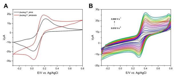
Fig. 6 (A) CVs of  $[Fe(CN)_6]^{3-}$  (1 mmol  $L^{-1}$ ) in KCl (0.1 mol  $L^{-1}$ ) on bare SPCE (black line) and SPCE/GCD (red line). (B) CVs of FcCAR (0.5 mmol  $L^{-1}$ ) in KCl (0.1 mol  $L^{-1}$ ) vs. the scan rate ( $\nu$ /V s<sup>-1</sup>) on SPCE/GCD.
