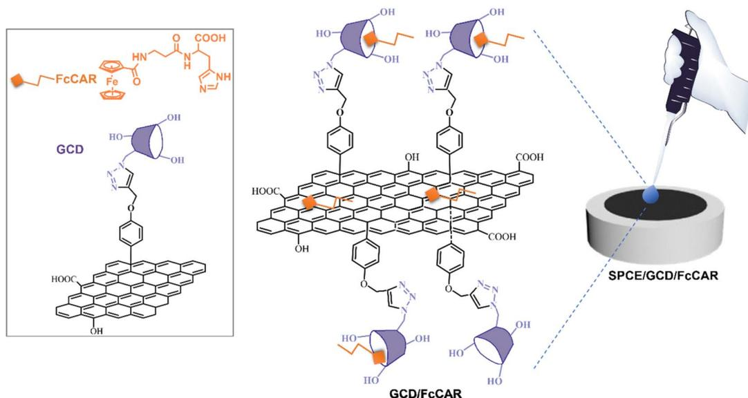
Fig. 1 Representative illustration of SPCEs modified with the nanoassembled GCD/FcCAR system. The chemical structures of GCD and FcCAR are shown on the left.
