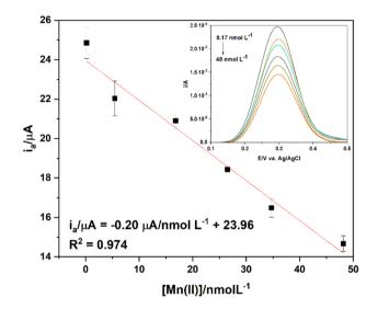
Fig. 7 Linear range of the anodic ( $i_a$ ) peak currents of FcCAR vs. Mn( $\shortparallel$ ) concentration (0.17  $\leq$  [Mn( $\shortparallel$ )]/nmol L<sup>-1</sup>  $\leq$  48) on SPCE/GCD. The inset shows the respective DPV scans.
