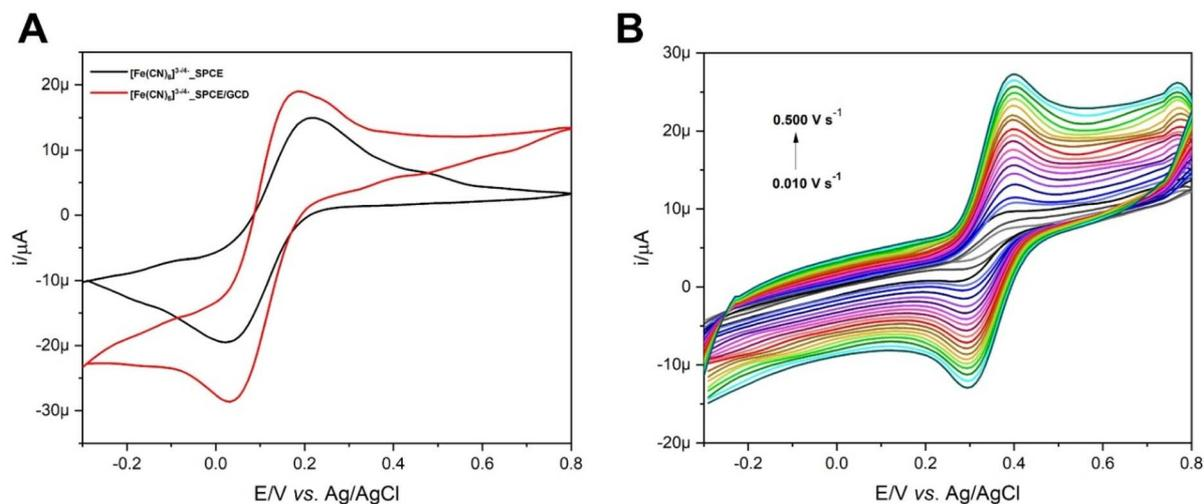
Fig. 6 (A) CVs of  $[\text{Fe}(\text{CN})_6]^{3-}$  ( $1 \text{ mmol L}^{-1}$ ) in  $\text{KCl}$  ( $0.1 \text{ mol L}^{-1}$ ) on bare SPCE (black line) and SPCE/GCD (red line). (B) CVs of FcCAR ( $0.5 \text{ mmol L}^{-1}$ ) in  $\text{KCl}$  ( $0.1 \text{ mol L}^{-1}$ ) vs. the scan rate ( $\nu/\text{V s}^{-1}$ ) on SPCE/GCD.
