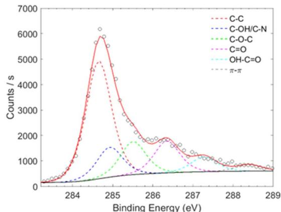
Fig. 3 XPS C 1s high resolution spectra of the GCD sample deconvoluted using six Gauss–Lorentzian functions.
