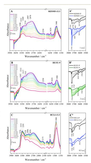
Fig. 4 FTIR difference spectra of  $NH_3$  adsorbed (max pressure 40 mbar) on hierarchical (A) HZSM5-13.3, (B) HUSY-9 and (C) HCLI-13.3 samples at room temperature. The intermediate pressures at which spectra are collected during desorption are reported in the figure. On the right, a comparison between the spectra of the desilicated samples and their corresponding parent samples in the OH stretching region (A'-C') is provided.
