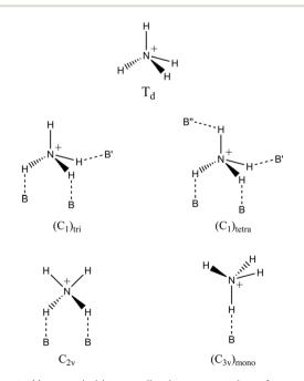
Scheme 1 Most probable coordination geometries of ammonium ions in zeolite environments.
