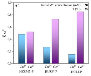
Fig. 9 Amount of  $Cu^{2+}$  and  $Co^{2+}$  concentrations captured by the studied zeolites from the multi-ion aqueous solution after 24 hours, expressed as (A)  $\mu$ mol g<sup>-1</sup> and (A')  $\chi_{M^{n+}}$ . The amount of BAS in 60 mg of material is also provided.
