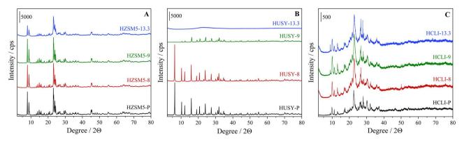
Fig. 1 XRD patterns of (A) HZSM5, (B) HUSY and (C) HCLI samples desilicated under different pH conditions
