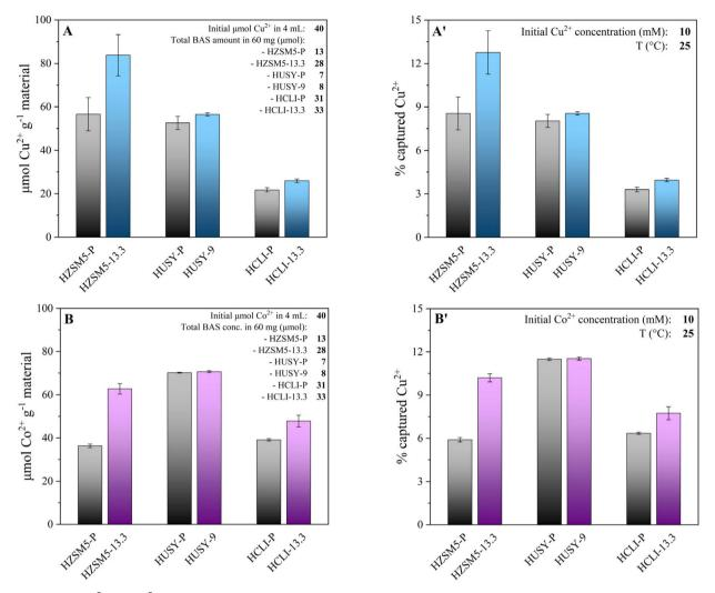
Fig. 8 Amounts of  $Cu^{2+}$  and  $Co^{2+}$  captured by the studied zeolites from their respective aqueous solutions after 24 hours, expressed as (A and B) umol q<sup>-1</sup> and (A' and B') percentage of the captured metal ion. The amount of BAS in 60 mg of material is also provided (the bars represent the mean values; the error bars indicate the standard deviations, calculated considering, for each sample, the triplicate sets of analyses performed on the two aliquots).
