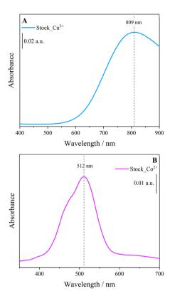
Fig. 7 UV-vis spectra of (A)  ${\rm Cu}^{2+}$  and (B)  ${\rm Co}^{2+}$  aquo complexes in solution. The spectra correspond to the stock solutions of the two metal ions ( $\sim$ 10 mM concentration) and are presented over the 400–900 nm range for  ${\rm Cu}^{2+}$  and the 350–700 nm range for  ${\rm Co}^{2+}$ , respectively.
