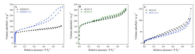
Fig. 2 N<sub>2</sub> adsorption/desorption isotherms at 77 K of (A) HZSM5, (B) HUSY and (C) HCLI desilicated under different pH conditions.
