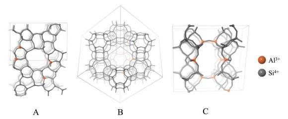
Scheme 2 Spatial distribution of Al<sup>3+</sup> atoms within the crystallographic unit cells of the zeolites (A) HZSM5; (B) HUSY and (C) HCLI.<sup>58</sup>
