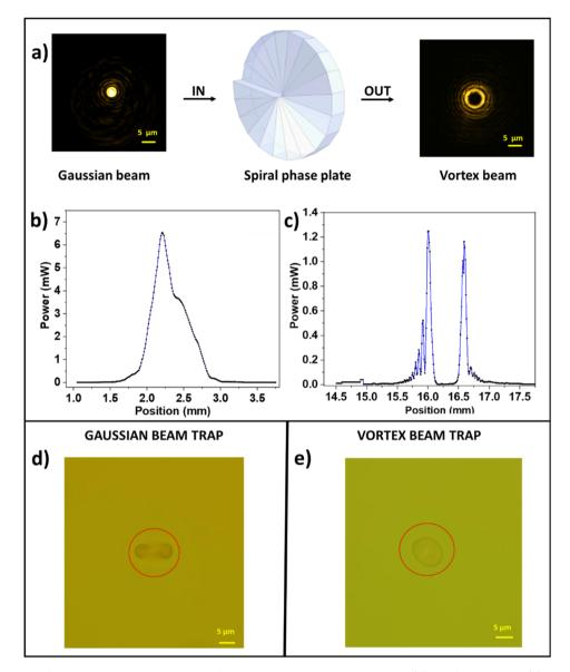
Fig. 2 (a) Conversion of Gaussian to vortex beam using SPP. The transverse beam profile of (b) the Gaussian and (c) the vortex laser beam. Optical image of live single RBC trapped using (d) Gaussian beam and (e) vortex beam.
