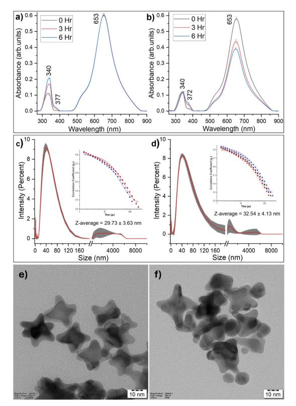
Fig. 3 Stability of AuNPs in saline using UV-vis and DLS measurements for as-prepared AuNPs (a and c) and AuNPs in saline (b and d). The insets in (c) and (d) show the cumulants fit for three trials. The TEM images of (e) as-prepared and (f) saline-treated AuNPs.
