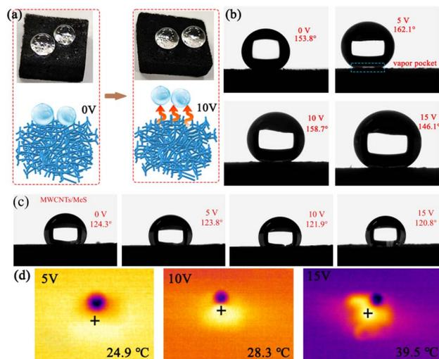
Fig. 5 The CA of ODT/MWCNTs/MeS electrodes under applied voltage. (a) The water droplet state on the electrode surface. (b) The CA of  $158.7^\circ$  with 0 V,  $162.1^\circ$  with 5 V,  $153.8^\circ$  with 10 V,  $146.1^\circ$  with 15 V. (c) The CA of MWCNTs/MeS electrode with 0 V, 5 V, 10 V, 15 V, respectively. (d) The thermal imaging of a droplet on the electrode surface under different supply voltages.
