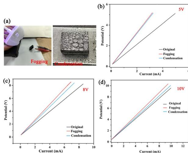
Fig. 7 (a) The photographs of original ODT/MWCNTs/MeS electrodes, fog humidification and condensation on the surface of electrodes. The  $C-V$  curves of ODT/MWCNTs/MeS electrodes at 5 V (b), 8 V (c), 10 V (d) external voltage and three wetting states.
