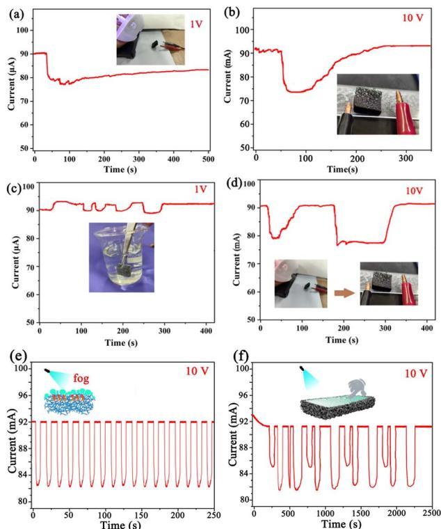
**Fig. 9** (a) The fogs condense on the surface of ODT/MWCNTs/MeS porous electrode. (b) After the droplets condense on the ODT/MWCNTs/MeS electrode, and the electrode is heated with a hair dryer. (c) The electrodes are soaked in hot water. (d) The fogs condense on the ODT/MWCNTs/MeS porous electrode with an external voltage of 10 V. (e) The fogs are intermittently sprayed onto the ODT/MWCNTs/MeS electrode at 10 V. (f) Pressing the ODT/MWCNTs/MeS electrode with a water film.
