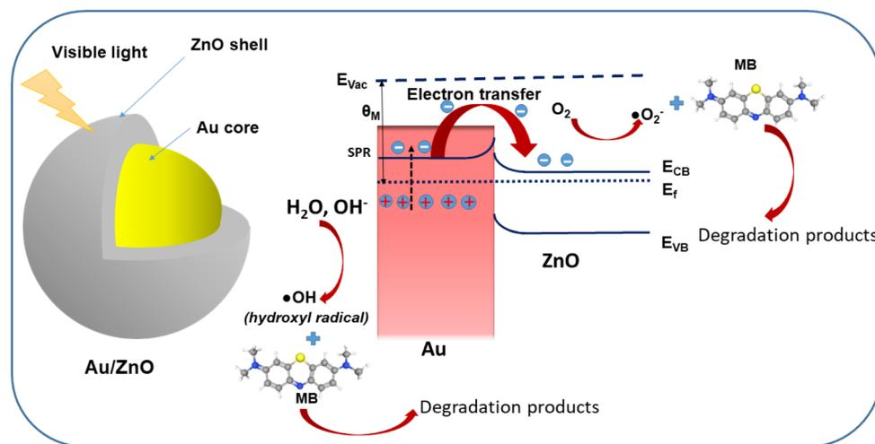
Fig. 7 Schematic diagram illustrating energy band alignment of reverse Au/ZnO core/shell nanostructures and proposed processes of generation of charge carriers, migration of the generated carriers and creation of reactive radicals for MB degradation.  $E_f$  = Fermi level,  $E_{CB}$  = conduction band of ZnO,  $E_{VB}$  = valence band of ZnO,  $E_{vac}$  = vacuum level.
