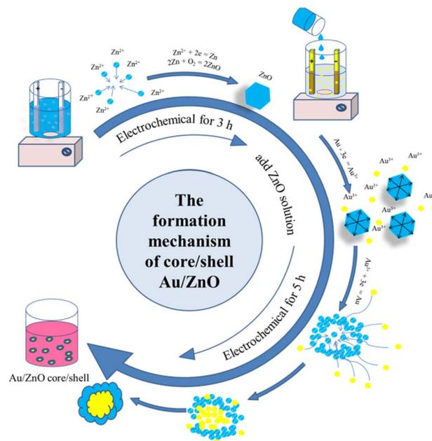
Fig. 4 The formation mechanics of reverse Au/ZnO core/shell nanostructures.
