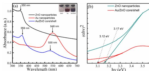
Fig. 1 (a) UV-vis absorption spectra of ZnO nanoparticles, gold nanoparticles and Au/ZnO core/shell nanostructures; (b) Tauc plots showing the bandgap energies.
