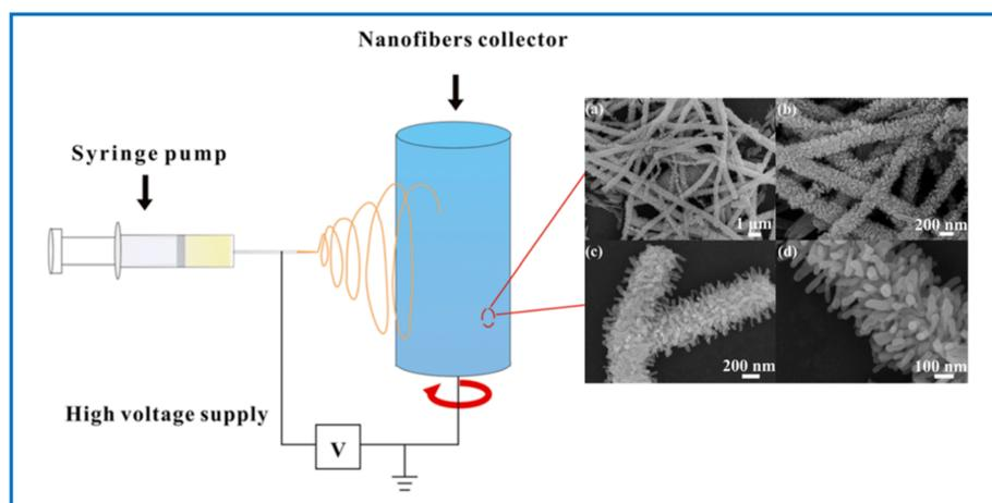
Fig. 5 Schematic diagram of electrospinning process for MO, synthesis FESEM images of the  $\alpha$ -Fe<sub>2</sub>O<sub>3</sub>/TiO<sub>2</sub> HSs: (a and b) panoramic and (c and d) magnified.<sup>73</sup> Permission Copyright © 2013, ACS.
