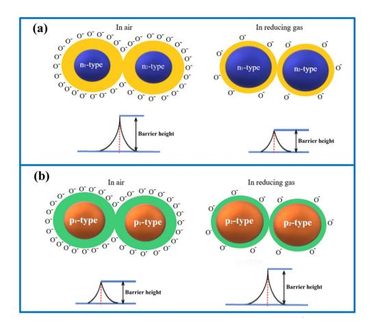
Fig. 7 Change in barrier height of (a) n-n HJ and (b) p-p HJ in the presence of air and reducing gas
