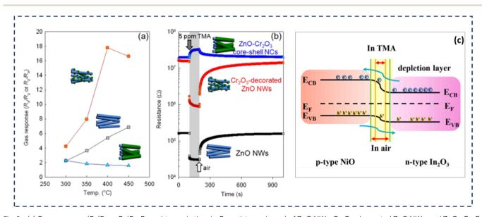
Fig. 8 (a) Gas responses  $(R_a/R_g \text{ or } R_g/R_a : R_a$ , resistance in the air;  $R_g$ , resistance in gas) of ZnO NWs,  $Cr_2O_3$ -decorated ZnO NWs, and ZnO- $Cr_2O_3$ core-shell NCs to 5 ppm TMA over the temperature range of 300-450 °C. (b) Dynamic sensing transients to 5 ppm TMA at the sensor temperature of 400 °C. $^{72}$  Permission Copyright © 2012, IOP. (c) The proposed energy band structure diagram for NiO-In $_2O_3$  HJs. $^{47}$  Permission Copyright © 2022, Elsevier.
