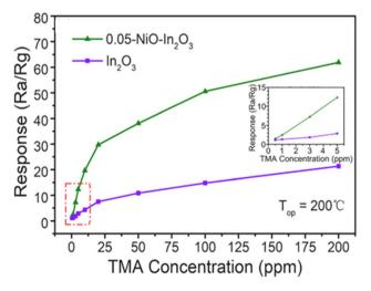
Fig. 10 The sensor exhibited responses to TMA concentrations ranging from 0.5 to 200 ppm TMA at 200  $^{\circ}$ C.<sup>47</sup> Permission Copyright © 2022, Elsevier.
