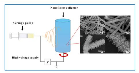
Fig. 5 Schematic diagram of electrospinning process for MO, synthesis FESEM images of the  $\alpha$ -Fe<sub>2</sub>O<sub>3</sub>/TiO<sub>2</sub> HSs: (a and b) panoramic and (c and d) magnified.73 Permission Copyright © 2013, ACS.
