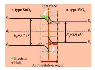
Fig. 9 Energy band diagram of the  $WO_3$ - $SnO_2$  (n-n) HJ at thermal equilibrium.
