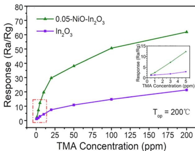
Fig. 10 The sensor exhibited responses to TMA concentrations ranging from 0.5 to 200 ppm TMA at 200 °C.<sup>47</sup> Permission Copyright © 2022, Elsevier.
