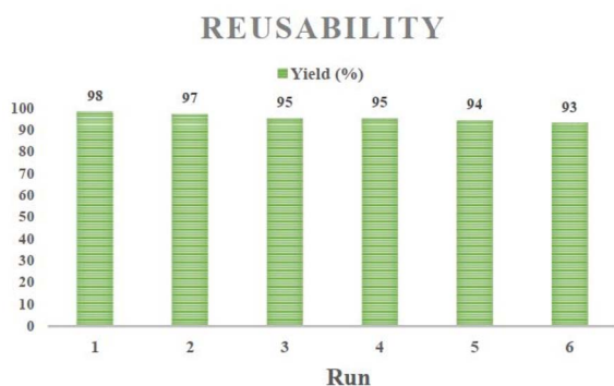
Fig. 12 The reusability results of the Co-Ni/Fe 3 O 4 @MMSHS nanocatalyst under the model reaction.
