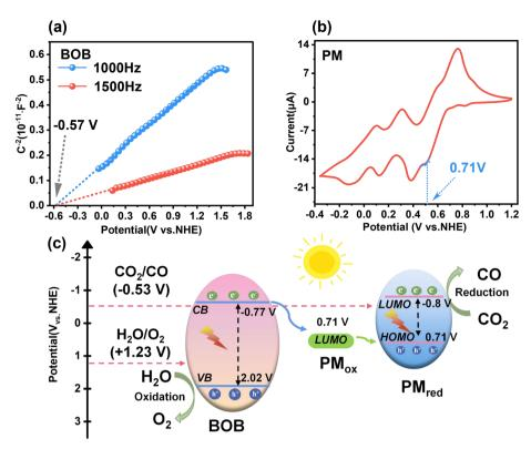
Fig. 6 (a) The M-S curve of BOB, (b) the CV curve of PM; and (c) the mechanism diagram of photocatalytic  $CO_2$  reduction reaction based on  $t_{200}$ -PM/BOB<sub>0.5</sub>.
