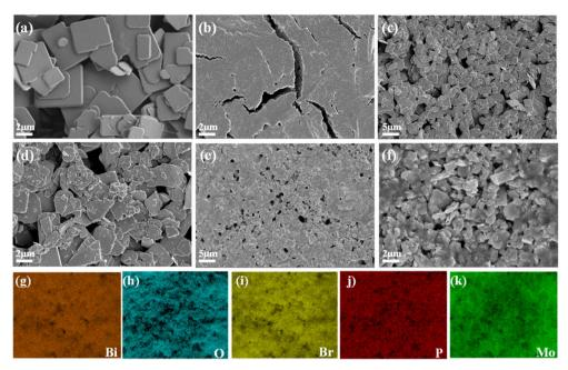
Fig. 1 SEM images of catalyst (a) BOB, (b) PM, (c and d)  $t_{25}$ -PM/BOB<sub>0.5</sub> and (e and f)  $t_{200}$ -PM/BOB<sub>0.5</sub>; (g-k) elements mapping of Bi, O, Br, P, and Mo in the corresponding region.
