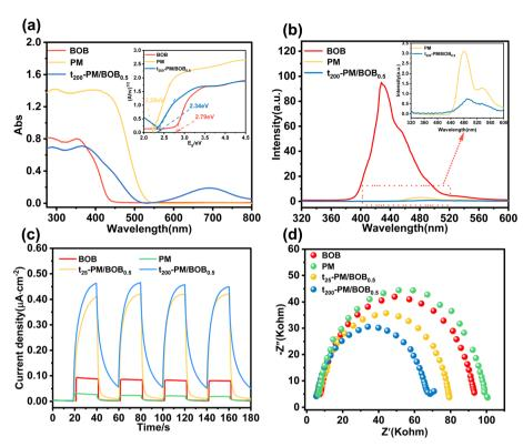
Fig. 4 (a) UV-vis DRS spectra of catalysts BOB, PM and  $t_{200}$ -PM/BOB<sub>0.5</sub>, with the band gap diagram of the corresponding catalyst illustrated; (b) solid PL spectra of BOB, PM and  $t_{200}$ -PM/BOB<sub>0.5</sub>, with amplified fluorescence spectra of PM and  $t_{200}$ -PM/BOB<sub>0.5</sub> shown in the embedded spectrogram; (c) photocurrent response and (d) EIS of BOB, PM,  $t_{25}$ -PM/BOB<sub>0.5</sub>, and  $t_{200}$ -PM/BOB<sub>0.5</sub>.
