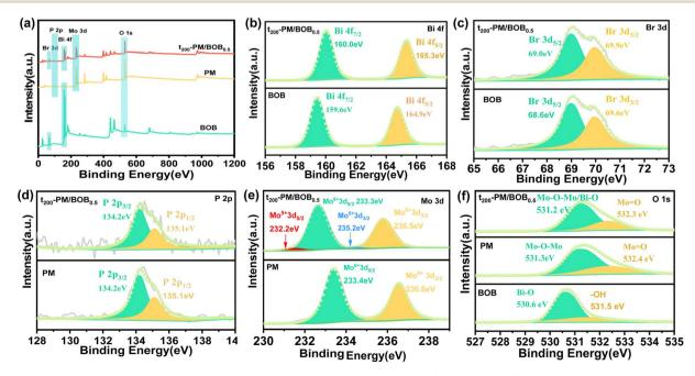
Fig. 3 (a) XPS survey spectrum and high-resolution XPS of (b) Bi 4f, (c) Br 3d, (d) P 2p, (e) Mo 3d and (f) O 1s in catalyst BOB, PM and t<sub>200</sub>-PM/ BOB<sub>0.5</sub>.
