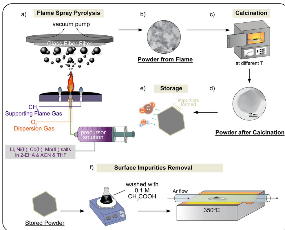
Fig. 1 Depiction of the  $\text{LiNi}_{1/3}\text{Mn}_{1/3}\text{Co}_{1/3}\text{O}_2$  (NMC) nanoparticle synthesis. Flame spray pyrolysis yields nanopowder (a and b), which is then calcined (c and d) to achieve a high-performance NMC nanopowder. The calcined powder inevitably encounters air exposure, which degrades the surface (e). Surface impurities can be removed *via* acid wash and subsequent drying (f).
