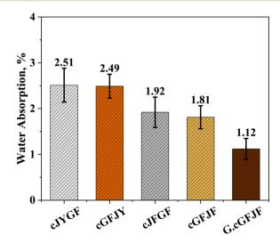
Fig. 8 Water absorbency of different wrapped and treated jute-glass hybrid composites.
