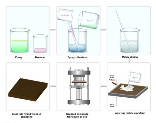
Fig. 3 Composite fabrication process.
