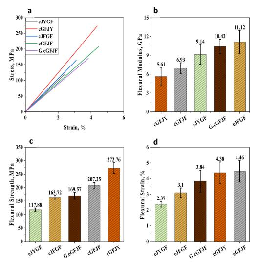
Fig. 6 (a) Flexural stress-strain curve, (b) flexural modulus, (c) flexural strength, (d) flexural strain of different wrapped and treated jute-glass hybrid composites
