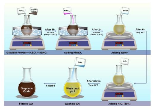
Fig. 1 Graphene oxide synthesis process
