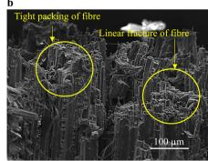
Fig. 9 (a) SEM fracture specimen of filed retted jute roving composite without GO coating at  $250 \times$  magnification, (b) SEM fracture specimen of field retted jute roving composites with GO coatings at  $250 \times$  magnification.
