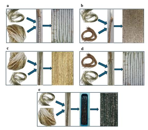
Fig. 2 Development hybrid wrapped roving: (a) raw jute in the core wrapped by glass fibre; (b) glass fibre in the core wrapped by commercial jute fibre; (c) glass fibre in the core wrapped by field retted jute fibre; (d) commercial yarn in the core wrapped by glass fibre and (e) dip coating of hybrid roving in the GO solution.
