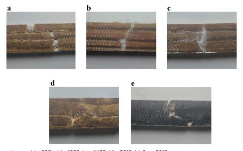
Fig. 4 Samples after tensile test: (a) cGFJY, (b) cJFGF, (c) cJYGF, (d) cGFJF, (e) G.c cGFJF.
