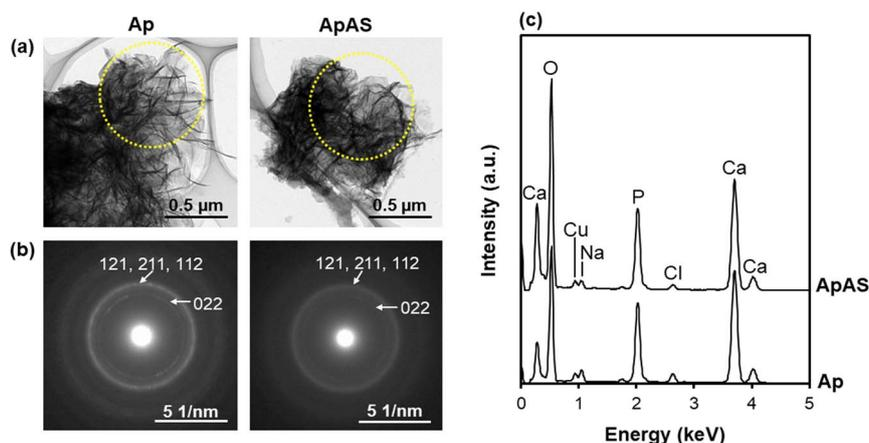
Fig. 4 (a) TEM images, (b) SAED patterns obtained from the circled regions in (a), and (c) STEM-EDX spectra of the precipitates collected from **Ap** and **ApAS**. The Cu peak in (c) is derived from the TEM grid.
