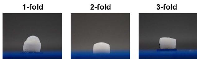
Fig. 6 Side view images of the **ApAS** sponge after drop-casting of the differently diluted (dilution factor: 1-fold, 2-fold, and 3-fold) dispersions (50  $\mu\text{L}$ ) of the CF-immobilized apatite particles.
