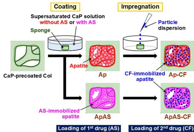
Fig. 1 Fabrication scheme of Ap, ApAS, Ap-CF, and ApAS-CF.
