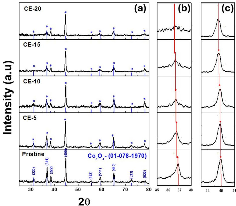
Fig. 1 (a) XRD patterns of  $\text{Co}_3\text{O}_4$  synthesized without rotten *Solanum melongena* juice (pristine) and with 5 mL (CE-5), 10 mL (CE-10), 15 mL (CE-15) and 20 mL (CE-20) of rotten *Solanum melongena* juice. (b) (311) plane peak shift of corresponding XRD patterns. (c) (400) plane main peak shift of corresponding XRD patterns.
