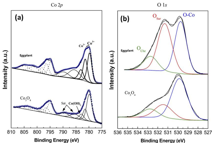
Fig. 4 X-ray core level spectra of pure  $\text{Co}_3\text{O}_4$  nanostructures and 15 mL rotten *Solanum melongena* juice mediated  $\text{Co}_3\text{O}_4$  nanostructures (a)  $\text{Co } 2p_{3/2}$ , (b)  $\text{O } 1s$ .
