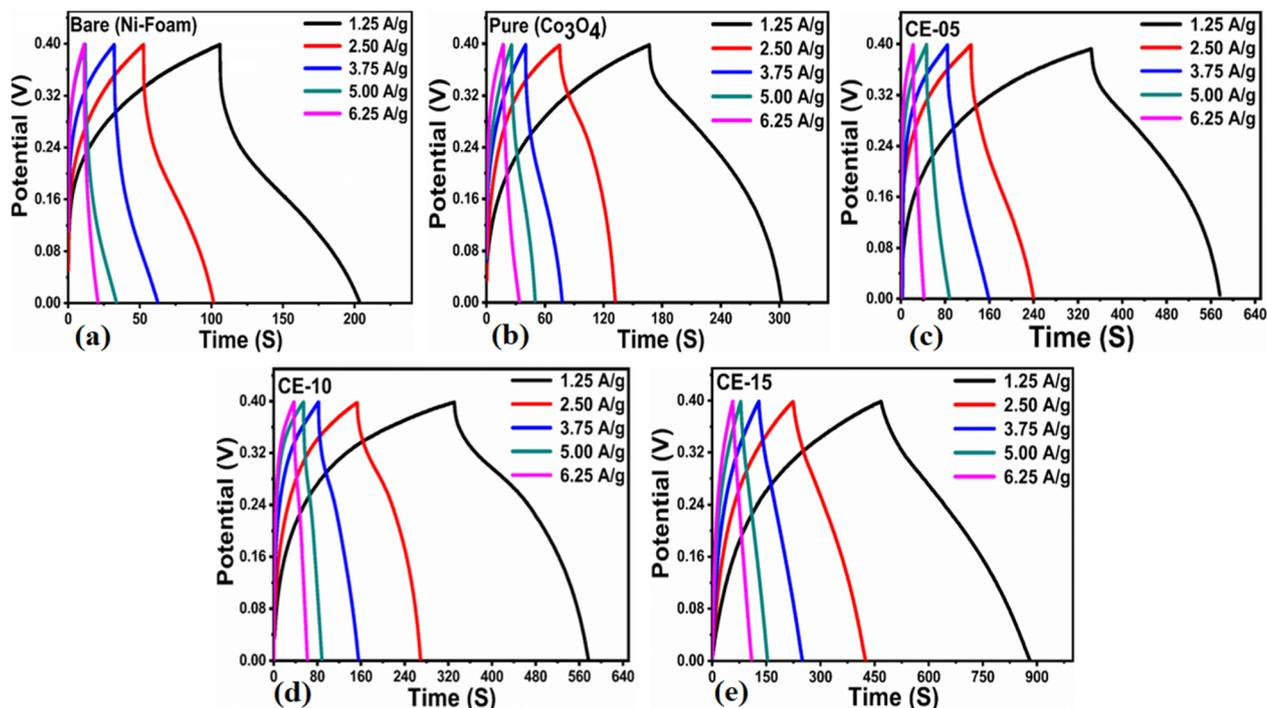
Fig. 7 (a–e)  $\text{Co}_3\text{O}_4$  nanostructures with different volumes and without rotten *Solanum melongena* juice (like CE-05, CE-10, CE-15, CE-20, CE stands for cobalt oxide-*Solanum melongena* juice) for the illustration of redox aspects using GCD curves at various current densities in 3.0 M KOH aqueous solution.
