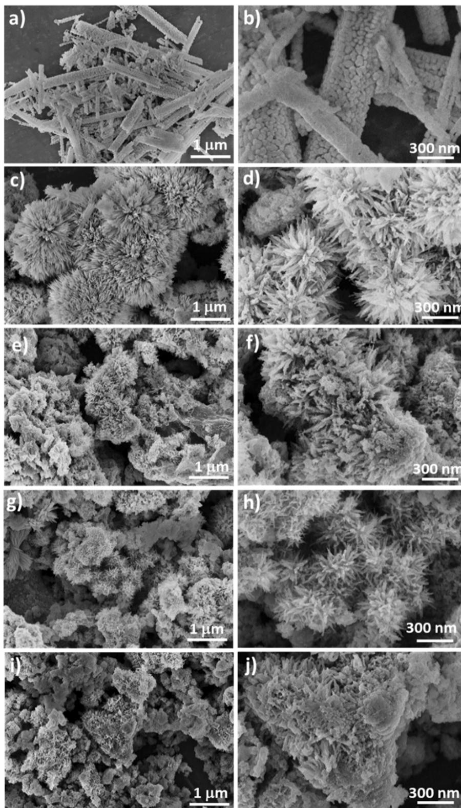
Fig. 2 SEM images at different magnifications of  $\text{Co}_3\text{O}_4$  synthesized (a and b) without rotten *Solanum melongena* juice and (c and d) with 5 mL, (e and f) 10 mL, (g and h) 15 mL and (i and j) 20 mL of rotten *Solanum melongena* juice.
