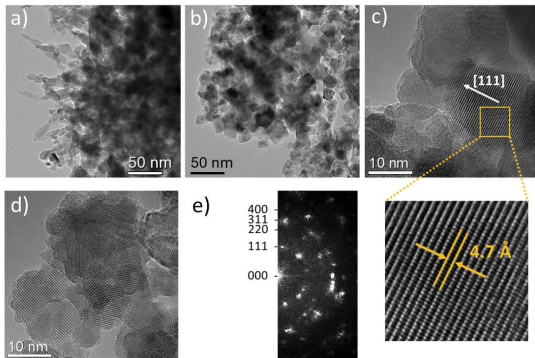
Fig. 3 (a and b) TEM and (c and d) HRTEM micrographs at different magnifications of  $\text{Co}_3\text{O}_4$  sample prepared with 15 mL of rotten *Solanum melongena* juice and (e) corresponding fast Fourier transform of (d).
