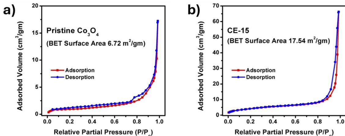
Fig. 5 BET surface area analysis of (a) pure  $\text{Co}_3\text{O}_4$  nanostructures and (b) 15 mL rotten *Solanum melongena* juice mediated  $\text{Co}_3\text{O}_4$  nanostructures.
