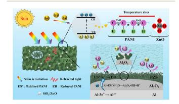
Fig. 8 Photothermal corrosion-resistant mechanism of the PZS coating.
