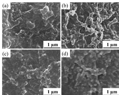
Fig. 2 SEM images of the composite coatings obtained with varying Ani : APS ratios (a) PZS-0.5, (b) PZS-1.0, (c) PZS-1.5, (d) PZS-2.0.
