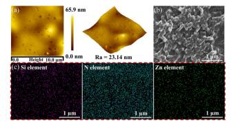
Fig. 4 Surface roughness and composition of the PZS-1.0 coating (a) surface roughness, (b) SEM and (c) the elemental distribution of N, Si and 7n
