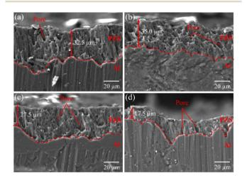
Fig. 3 Cross-sectional SEM images of different PZS composite coatings: (a) PZS-0.5, (b) PZS-1.0, (c) PZS-1.5, (d) PZS-2.0.
