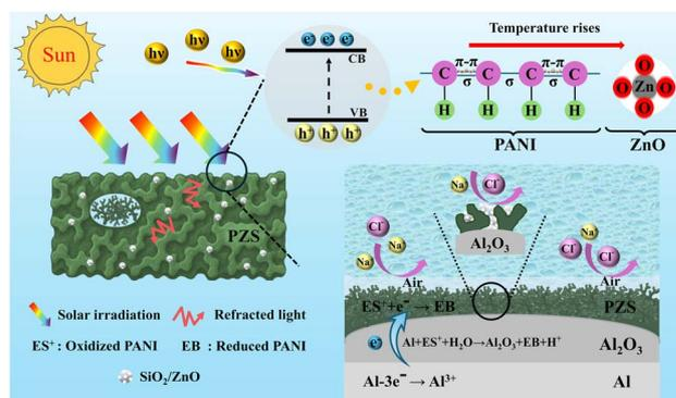
**Fig. 8** Photothermal corrosion-resistant mechanism of the PZS coating.**Table 2** Equivalent circuit fitting parameters
