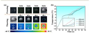
Fig. 6 Freezing/thawing behavior of water droplet on PZS coating (a) thermographic images, (b) temperature—time curves (The inset is magnified view).
