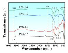
Fig. 1 The FT-IR spectra of the PZS samples.
