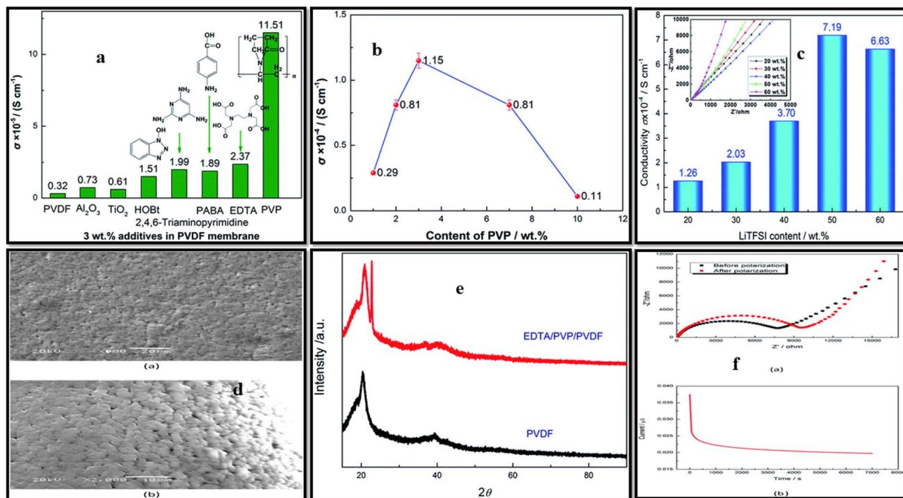
**Fig. 13** (a) Conductivity of different additives added to the PVDF, (b) effect of PVP content on conductivity, (c) effect of various compositions of LITFSI salt on the EDTA/PVP/PVDF membrane conductivity, (d) SEM micrographs at 900 $\times$  (a) and 2000 $\times$  (b) of EDTA/PVDF/PVP membrane, (e) XRD profiles of pristine PVDF and membrane, (f) EIS before and after polarization (a) and current vs. time plot during the polarization process (b).<sup>162</sup>
