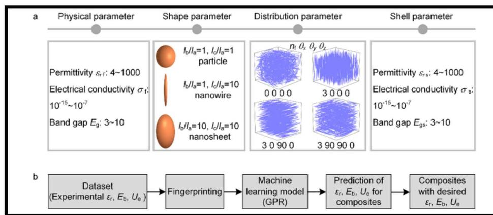
Fig. 22 ML workflow. (a) Schematic fingerprint representation of composites with various schemes of fillers doping. (b) Schematic of ML workflow for predicting  $\epsilon_r$ ,  $E_b$ , and  $U_e$ . Reproduced with permission from ref. 198.
