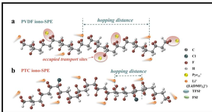
Fig. 19 Schematic illustration of  $\text{Li}^+$  transport mechanism in (a) PVDF-iono SPE versus (b) PTC-iono SPE. Key observations: In the PVDF system (a), the occupation of transport sites by  $\text{Pyr}_{13}^+$  cations increase the effective hopping distance for  $\text{Li}^+$  migration. The PTC system (b) demonstrates more efficient  $\text{Li}^+$  conduction pathways along polymer chains. Reproduced with permission from ref. 190.
