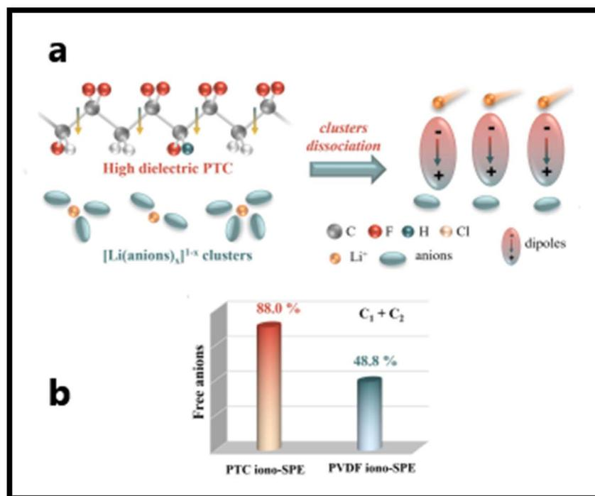
Fig. 20 (a) Schematic illustration of  $[\text{Li}(\text{anion})_x]^{1-x}$  cluster dissociation facilitated by high-dielectric-constant PTC. (b) Comparative ratio of free anions in PTC-iono-based SPE and PVDF-iono-based SPE, as quantified by Raman spectroscopy analysis. Reproduced with permission from ref. 190.
