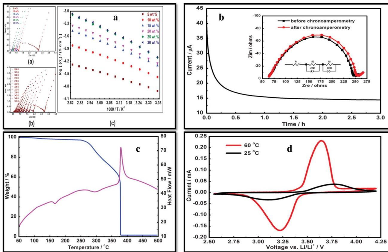
Fig. 11 (a) AC plots (a) various concentrations of LiFTSI salt, (b) 5 wt% LiFTSI salt at various temperatures, (c) temperature-dependent ionic conductivity at various salt concentrations. (b) CA and EIS analysis to find the  $t_+$  value (c) DSC and TGA thermograms with 20 wt% LiFTSI. (d) CV of LiFePO<sub>4</sub>/SPE/Li battery at 25 °C (black) and 60 °C (red). Reproduced with permission from ref. 112.
