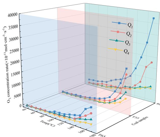
Fig. 3 Three-dimensional curve of the  $O_2$  consumption rate.
