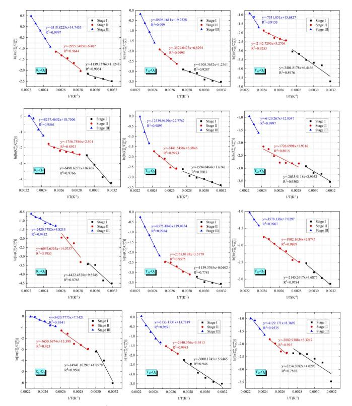
Fitted relationship between  $ln[ln(C_{O_2}^{in}/C_{O_2}^{out})]$  and 1/T in different reaction stages.
