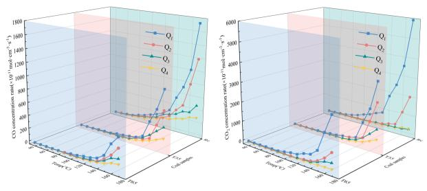
Fig. 4 Three-dimensional curve of carbon and oxygen gas generation rate
