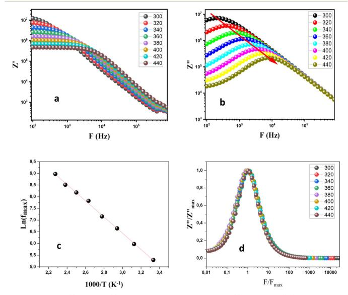
Fig. 6 Variation of the real (a) and imaginary (b) parts of the impedance as function of frequency, (c) the variation of ln(f<sub>max</sub>) as a function of 1000/ T, and (d) The scaling behavior of Z''/Z'.
