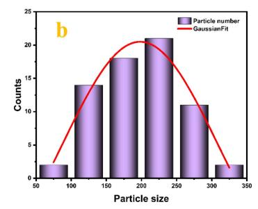
Fig. 2 (a) SEM image for Li Sr<sub>0.8</sub>Fe<sub>0.1</sub>Ni<sub>0.1</sub>PO<sub>4</sub> sample, (b) particles size distribution.
