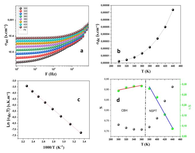
Fig. 5 (a) Evolution of conductivity *versus* frequency, (b) variation of  $\sigma_{dc}$  *versus*. Temperature, (c)  $Ln(\sigma_{dc})$  as function of 1000/T and (d) variation of s exponent as function of temperature.
