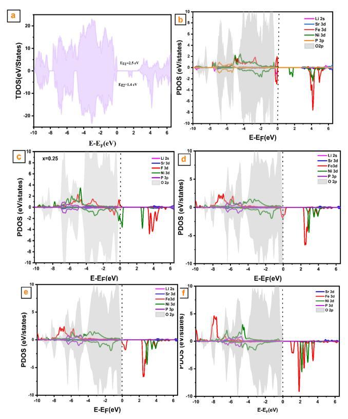
Fig. 3 Spin polarized calculated DOS) of  $\text{Li}_{1-x} \text{Sr}_{0.8} \text{Fe}_{0.1} \text{Ni}_{0.1} \text{PO}_4$ : total DOS (a) partial DOS of  $\text{Li}_{1-x} \text{Sr}_{0.8} \text{Fe}_{0.1} \text{Ni}_{0.1} \text{PO}_4$ , ((b) x=0, (c) x=0.25, (d) x=0.5, (e) x=0.75, and (f) x=1.
