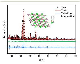
Fig. 1 Rietvield refinement of X-ray diffraction data for the  $LiSr_{0.8}$ - $Fe_{0.1}Ni_{0.1}PO_4$  powder sample. The inset of figure presents the crystal structure of  $LiSr_{0.8}Fe_{0.1}Ni_{0.1}PO_4$ .
