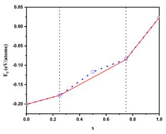
Fig. 10 The estimated Ef values for  $\text{Li}_{(1-x)}\text{Fe}_{0.1}\text{Ni}_{0.1}\text{Sr}_{0.8}\text{PO}_4$  system as a function of concentration x. Data points located on the convex hull (solid red line) denotes stability against any type of decomposition. Metastable phases are represented by open circles on the blue dotted line. The concentration x is expressed in formula units (fu). x=1 implies 32 Li atoms removed, respectively.
