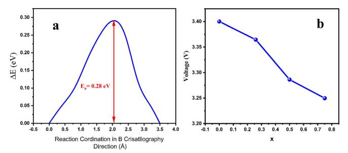
Fig. 9 (a) Plots of Li diffusion activation barrier along B-crystallographic axis for (LiSr<sub>0.8</sub>Fe<sub>0.1</sub>Ni<sub>0.1</sub>PO<sub>4</sub>), (b) deintercalation potentials (V) for Li<sub>1...</sub>Fe<sub>0.1</sub>Ni<sub>0.1</sub>Sr<sub>0.8</sub>PO<sub>4</sub> (x = 0, 0.25, 0.5, 0.75).
