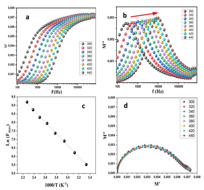
Fig. 8 Variation of the real (a) and imaginary (b) parts of the modulus, (c) the variation of  $ln(f_{max})$  as a function of 1000/T, and (d) the scaling behavior of M''/M'.
