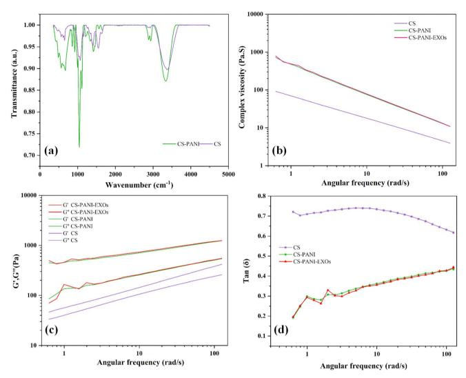
Fig. 2 (a) FTIR spectra of CS and CS-PANI hydrogels. (b) Complex viscosity of CS and CS-PANI hydrogels as a function of angular frequency. (c) Storage modulus (G') and loss modulus (G'') of CS and CS-PANI hydrogels across a range of angular frequencies. (d) Tan( $\delta$ ) vs. angular frequency of CS, CS-PANI, and CS-PANI-EXOs hydrogels.
