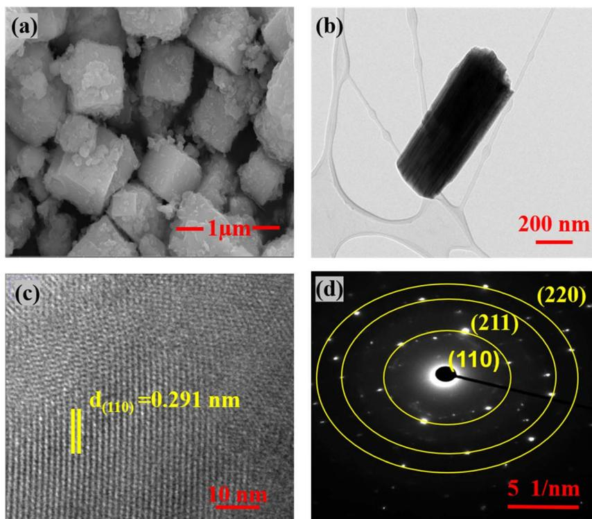
Fig. 2 (a) FE-SEM image of BSO with cubic morphology, (b) TEM image of BSO, (c) HRTEM with  $d$ -spacing 0.29 nm, and (d) SAED image of BSO.
