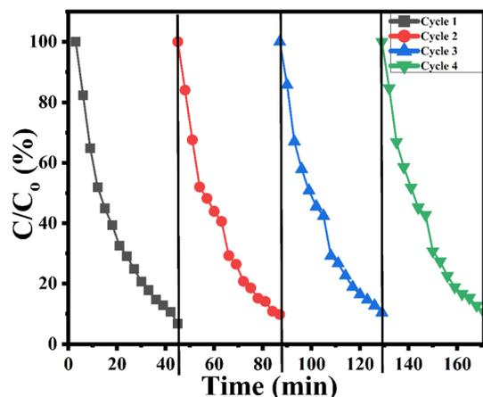
Fig. 13 Recyclability test of BSO photocatalyst, experimental conditions: [TC] = 0.01 g L<sup>-1</sup>, BSO = 0.4 g L<sup>-1</sup>, and volume: 80 ml.
