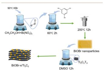
Scheme 1 Schematic of the preparation of BiOBr/Ti<sub>3</sub>C<sub>2</sub>.
