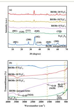
Fig. 2 (a) XRD patterns and (b) FT-IR spectra of BiOBr,  $Ti_3C_2T_x$  and BiOBr-x/Ti<sub>3</sub>C<sub>2</sub>.
