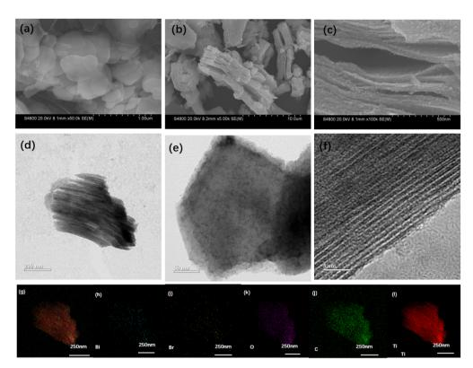
Fig. 1 SEM images of (a) BiOBr, (b) Ti<sub>3</sub>C<sub>2</sub>T<sub>x</sub> and (c) BiOBr-10/Ti<sub>3</sub>C<sub>2</sub>; (d) TEM and magnified TEM (e) images of BiOBr-10/Ti<sub>3</sub>C<sub>2</sub>; (f) HRTEM image of BiOBr-10/Ti<sub>3</sub>C<sub>2</sub>; elemental mapping images of (g) overall distribution, (h) Bi, (i) Br, (j) C, (k) O and (l) Ti in BiOBr-10/Ti<sub>3</sub>C<sub>2</sub>.
