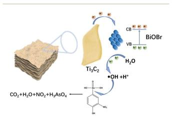
Scheme 2 Proposed mechanism for the photocatalytic degradation of roxarsone over  $\text{BiOBr/Ti}_3\text{C}_2.$
