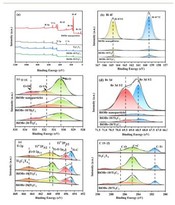
Fig. 3 (a) XPS survey spectra; high-resolution XPS spectra of (b) Bi 4f, (c) O 1s, (d) Br 3d, (e) Ti 2p and (f) C 1s for BiOBr,  $Ti_3C_2T_x$  and BiOBr- $x/Ti_3C_2$ .
