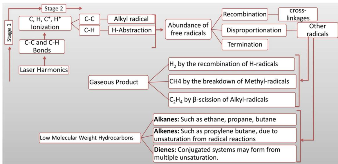
Fig. 5 The hypothetical laser-induced HDPE pyrolysis products.
