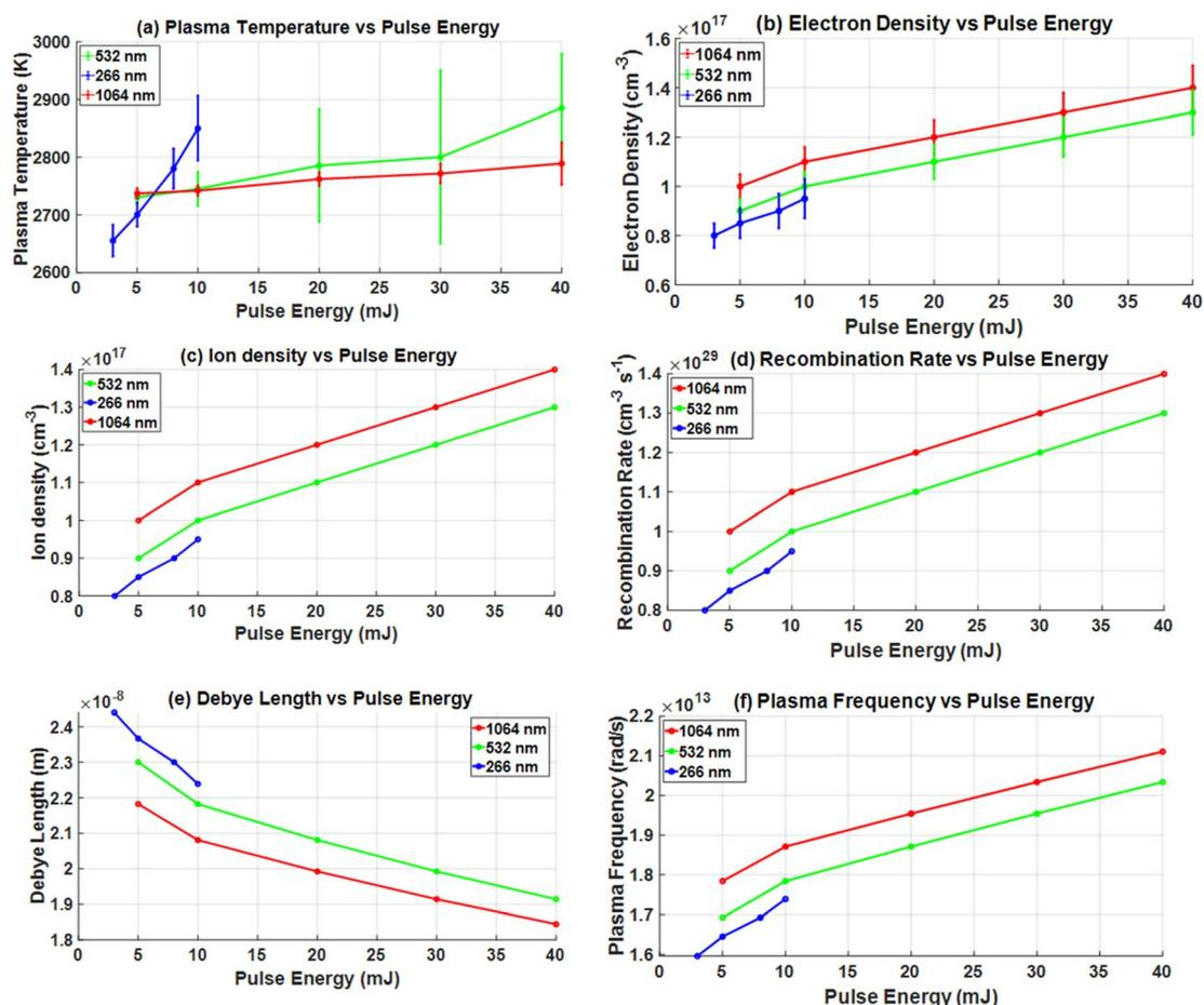
Fig. 8 Plasma parameters as a function of pulse energy: (a) temperature, (b) electron density, (c) ion density, (d) recombination rate, (e) Debye length, (f) and plasma frequency.
