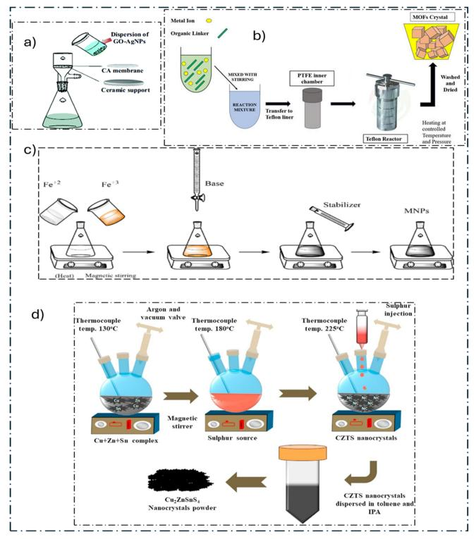
Fig. 3 (a) Vacuum filtration method,84 (b) hydrothermal/solvothermal technique,83 (c) co-precipitation method,84 and (d) hot injection method.85
