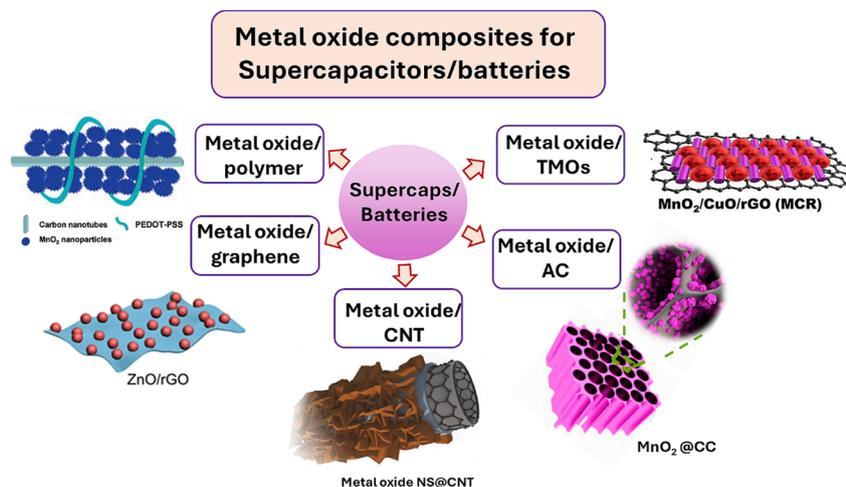
Fig. 4 Illustration of several forms of metal composite-based electrode materials for energy storage.<sup>95</sup>
