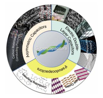
Fig. 1 Schematic of the commonly used electrode materials for various supercapacitor types. Asymmetric capacitors combine carbon materials with conducting polymers or metal oxides, while pseudocapacitors utilize metal oxides and conducting polymers. Graphene, carbon aerogels, activated carbons, carbon fibers, and carbon nanotubes are predominantly employed in EDLCs.31
