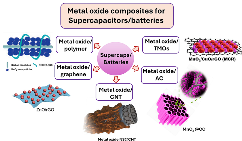
Fig. 4 Illustration of several forms of metal composite-based electrode materials for energy storage. 95
