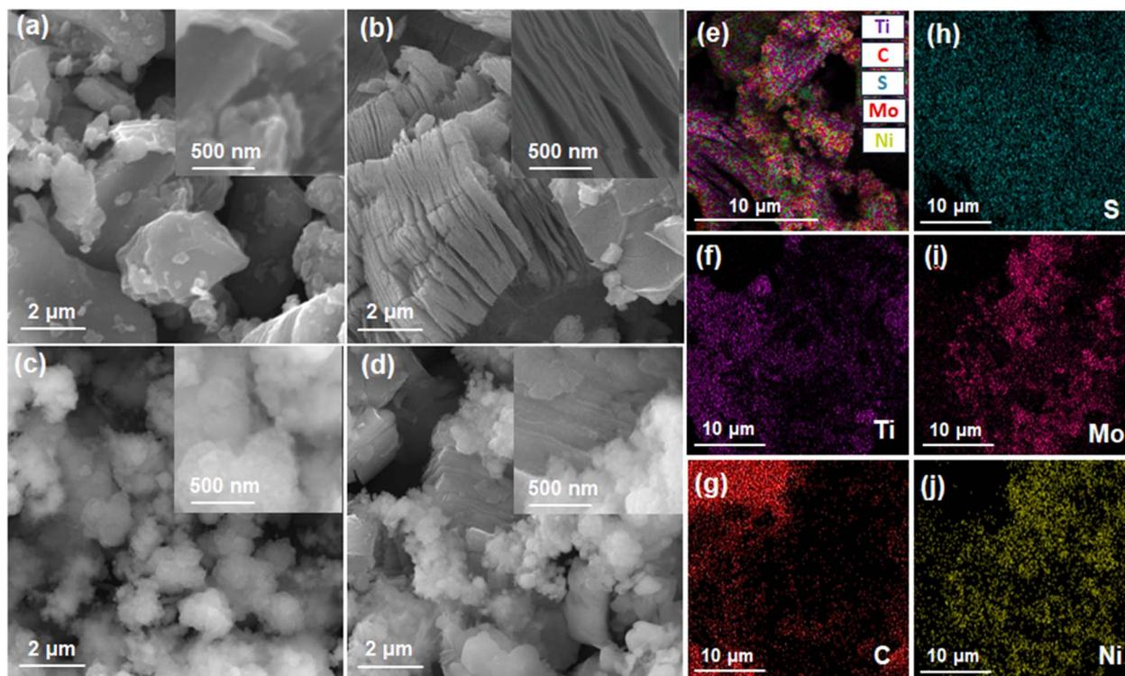
Fig. 1 SEM images of (a) titanium aluminium carbide MAX phase, (b)  $\text{Ti}_3\text{C}_2\text{T}_x$  MXene synthesized by etching of the MAX phase, (c)  $\text{NiMo}_3\text{S}_4$ , and (d)  $\text{NiMo}_3\text{S}_4$ -MXene and (e–j) EDS mapping of  $\text{NiMo}_3\text{S}_4$ -MXene.
