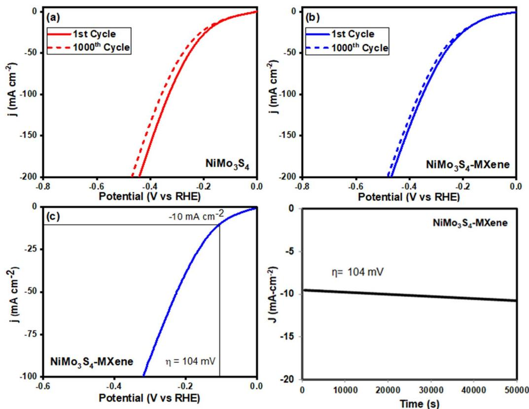
Fig. 7 LSV curves of electrocatalysts before and after 1000 cycles. (a) NiMo<sub>3</sub>S<sub>4</sub> and (b) NiMo<sub>3</sub>S<sub>4</sub>-MXene. (c) LSV of NiMo<sub>3</sub>S<sub>4</sub>-MXene and (d) chronoamperometry data of NiMo<sub>3</sub>S<sub>4</sub>-MXene.
