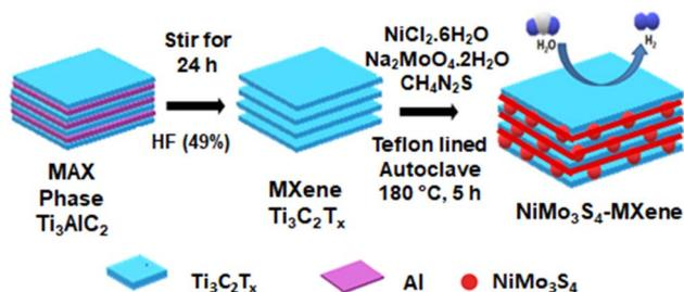
Scheme 1 Preparation of the NiMo<sub>3</sub>S<sub>4</sub>-MXene hybrid electrocatalyst.
