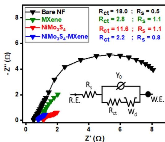
Fig. 6 Nyquist plot of bare Ni-foam, MXene, NiMo<sub>3</sub>S<sub>4</sub>, and NiMo<sub>3</sub>S<sub>4</sub>-MXene measured at a potential of -0.2 V vs. RHE (the unit of *R*<sub>ct</sub> and *R*<sub>s</sub> values is Ω).
