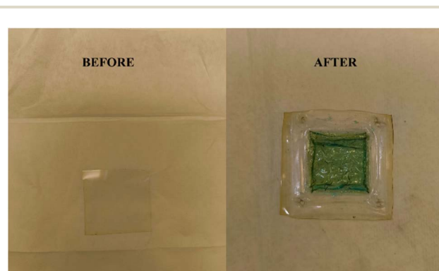
Fig. 16 The physical condition of NAFION, a proton-exchange membrane, before and after the evaluation of charge–discharge characteristics of VRFB for numerous cycles under varying operational conditions.
