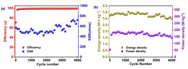
Fig. 8 (a) Efficiency and ESR and (b) energy and power density values of PCX40-based EDLC over 4000 charge-discharge cycles.
