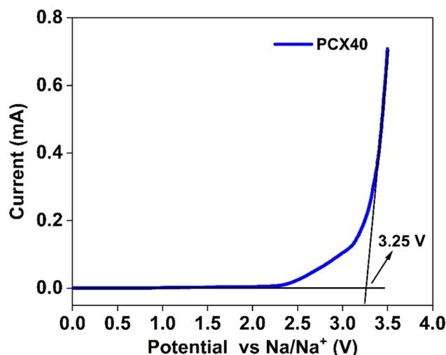
Fig. 5 LSV plot of optimum conducting sample of PCX40 SPE.
