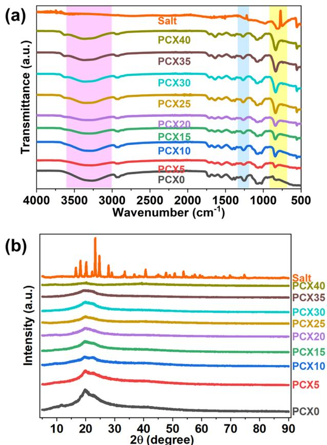
Fig. 2 (a) FTIR spectra of PVA/CS–NaPF<sub>6</sub> SPEs and NaPF<sub>6</sub> along with (b) XRD spectra of PVA/CS–NaPF<sub>6</sub> SPEs along with XRD spectra of NaPF<sub>6</sub> salt.
