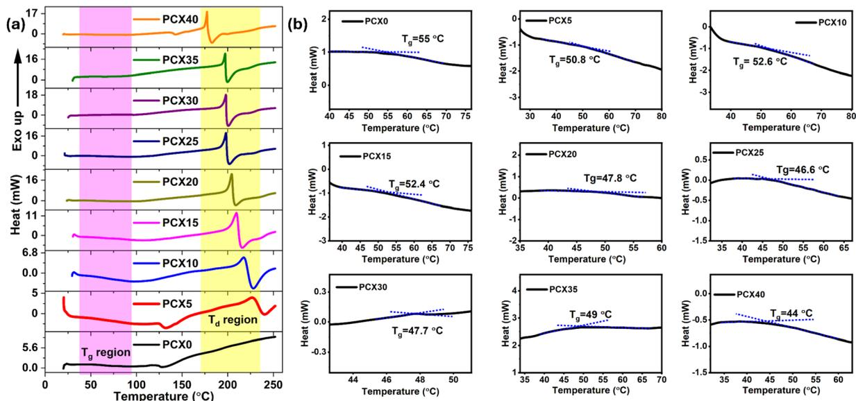
Fig. 4 (a) DSC thermogram illustrating glass transition region and thermal decomposition regions and (b) glass transition temperature variation in PVA/CS–NaPF<sub>6</sub> SPEs.
