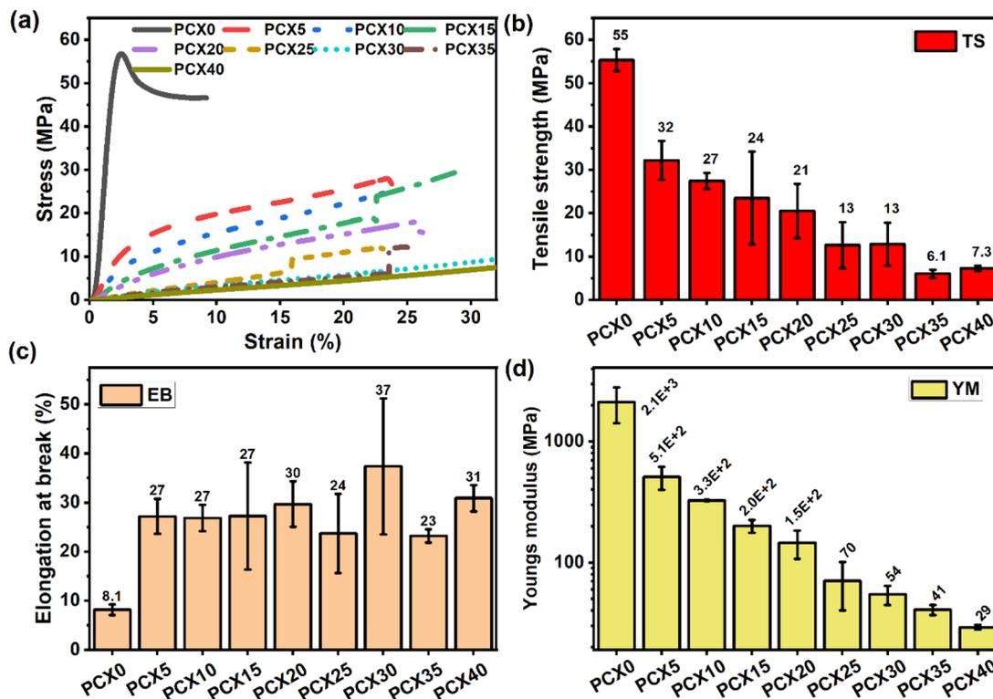
Fig. 6 (a) Stress–strain graph and (b)–(d) variation of the mechanical parameters for PVA/CS–NaPF<sub>6</sub> SPEs.
