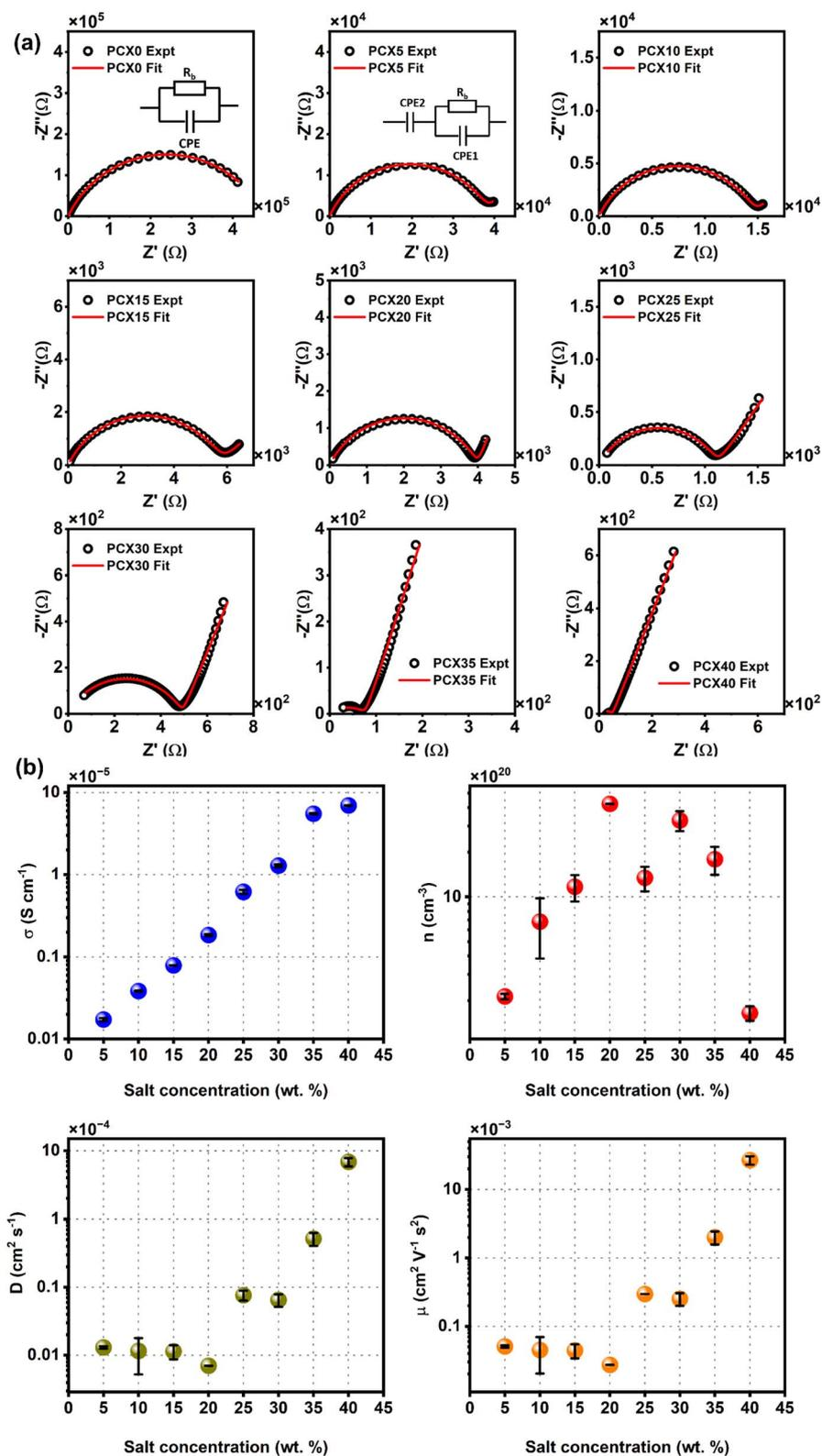
Fig. 3 (a) Nyquist plot of PVA/CS-NaPF<sub>6</sub> SPEs along with corresponding EEC which is used to fit it (inset) and (b) variation of ion transport properties as per S-G model along with bulk conductivity  $\sigma$  for PVA/CS-NaPF<sub>6</sub> SPEs.
