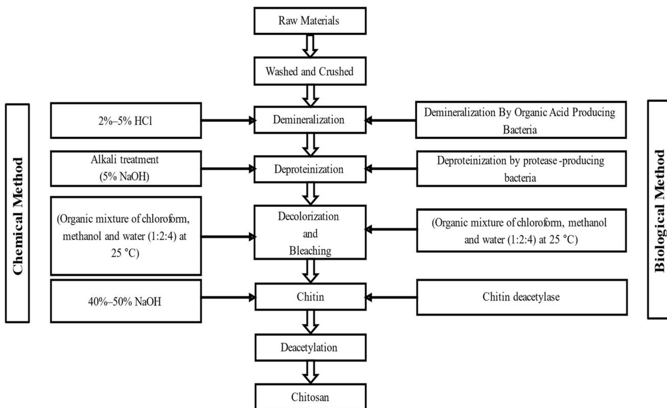
Fig. 3 Flow sheet of the extraction process of chitin and chitosan.<sup>8,79</sup>
