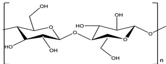
Fig. 4 Chemical structure of cellulose.<sup>180</sup>
