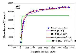
Fig. 12 (a) M–H hysteresis loop and LAS approach of saturation magnetization for the prepared perovskite. (b) M–H hysteresis loop and LAS approach of saturation magnetization for the prepared perovskite.
