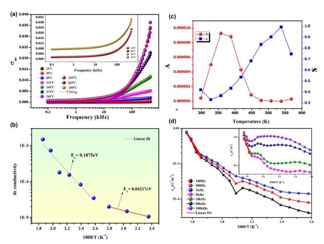
Fig. 10 (a) AC conductivity as a function of frequency at various temperatures with Jonscher Power law fitting. (b) DC conductivity vs. 1000/T. (c) Temperature-dependent s and A. (d) AC conductivity vs. 1000/T.
