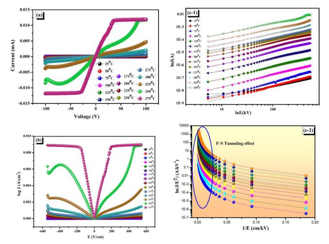
Fig. 13 (a) I-V-characteristic plot at various temperature. (b) Log J vs. E plot at various temperature. (c-1) Log J vs. log E plot at various temperature. (c-2) Log  $J/E^2$  vs. E plot at various temperature.
