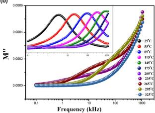
Fig. 9 (a) Variation of real modulus (M') with frequency at different temperatures. (b) Variation of imaginary modulus (M'') with frequency at different temperatures.
