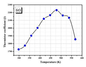
Fig. 11 (a and b): (a) Change in resistance with temperature; (b)  $\ln R$  versus 1/T (c) Thermistor constant ( $\beta$ ) vs. temperature.
