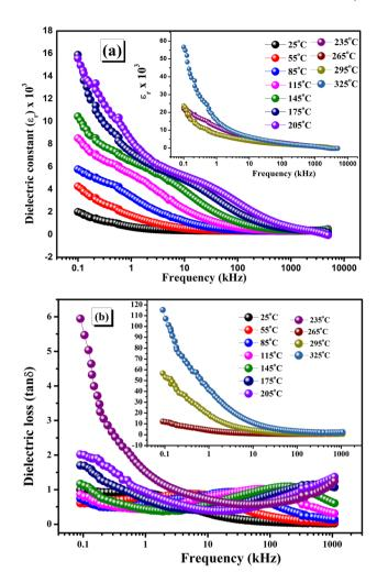
Fig. 6 (a) Frequency-dependent dielectric constant  $(\varepsilon_r)$  at different temperatures. (b) Frequency-dependent dielectric loss at various temperature.
