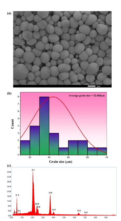
Fig. 2 (a) Microstructural analysis through FESEM micrograph of BCFZO. (b) Histogram mapping for the grain size of the sample. (c) Surface elemental composition by energy dispersive X-ray Spectroscopy.
