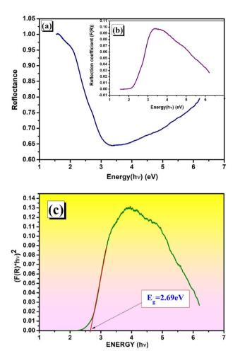
Fig. 5 (a) and (b): Typical UV-visible reflection spectra of synthesized BCFZO (a) reflectance vs. photon energy, (b) reflection coefficient vs. photon energy. (c) The calculated band gaps of the synthesized BCFZO using UV-vis reflection spectrum  $(F(R)*h\nu)^2 vs.$  photon energy.
