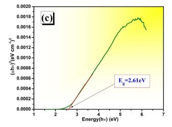
Fig. 4 (a) and (b): UV-vis spectroscopy (a) absorbance vs. wavelength, (b) absorption coefficient vs. photon energy. (c) The calculated band gaps of the synthesized BCFZO using UV-vis absorption spectrum.
