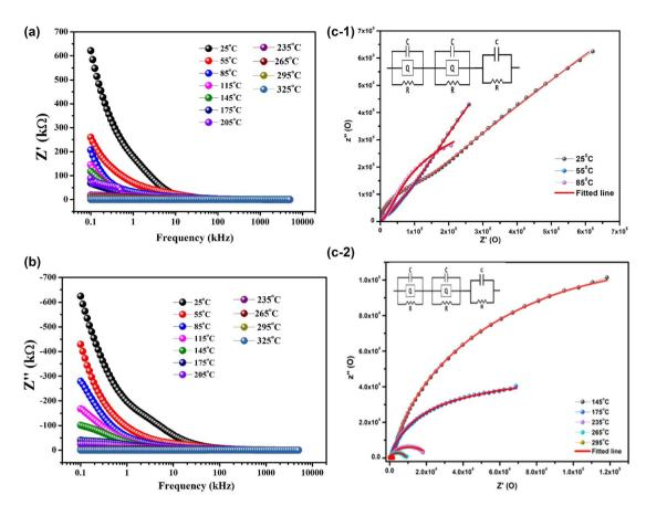
Fig. 8 (a) Frequency varying Real impedance (Z'). (b) Frequency varying imaginary impedance (Z'') with different temperature. (c-1) Z'-Z'' (impedance Nyquist plot) at lower temperature. (c-2) Z'-Z'' (impedance Nyquist plot) at higher temperature.
