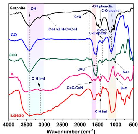
Fig. 1 FT-IR spectra of four components (graphite, GO, SGO, and IL) and IL@SGO.
