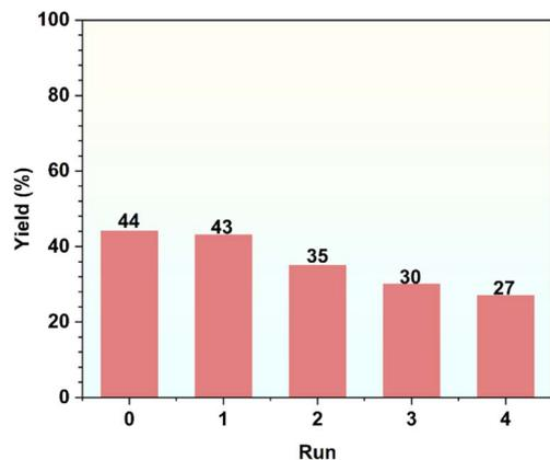
Fig. 9 Reusability of IL@SGO through catalysis in the synthesis process of 4aa.
