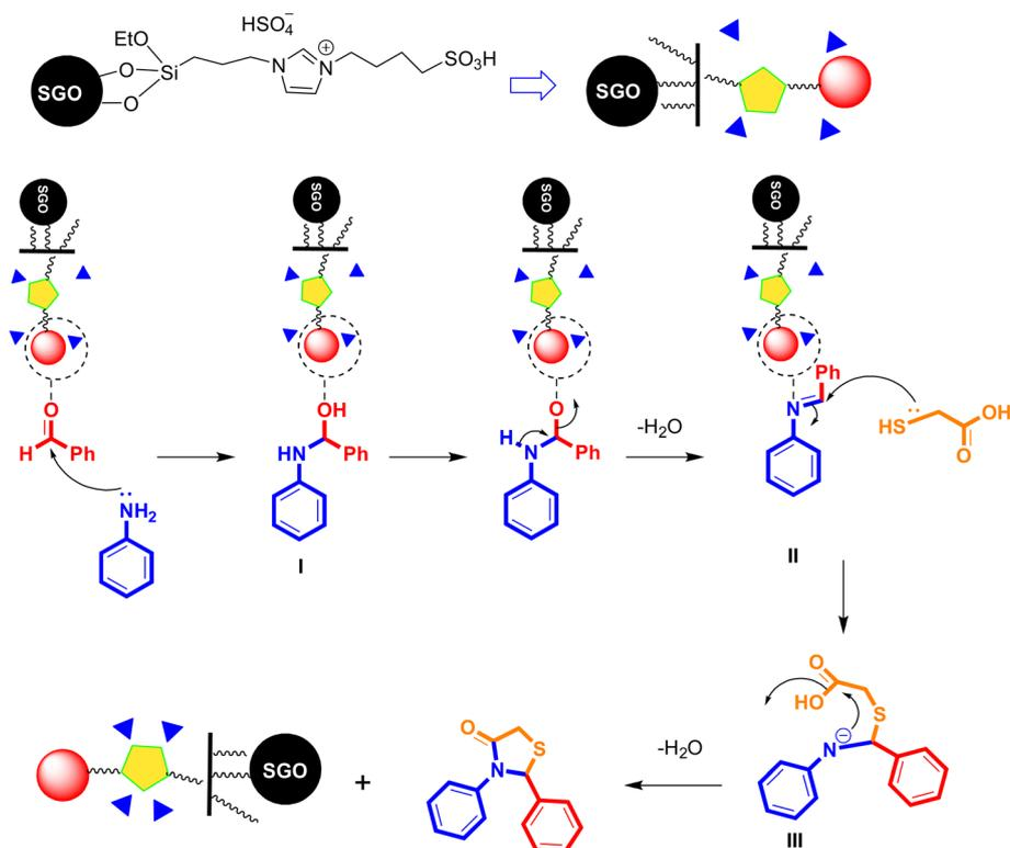
Scheme 4 Proposed reaction mechanism for the synthesis of **4aa**.
