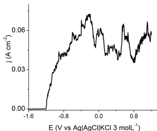
Fig. 1 Linear voltammogram of 0.005 mol L<sup>-1</sup> of NaNH<sub>4</sub>HPO<sub>4</sub>·4H<sub>2</sub>O at pH 7.5. Working electrode Mg plate, auxiliary electrode Pt wire, and reference electrode Ag|AgCl|KCl 3 mol L<sup>-1</sup>, at 0.1 mV s<sup>-1</sup>. Starting from open circuit potential.
