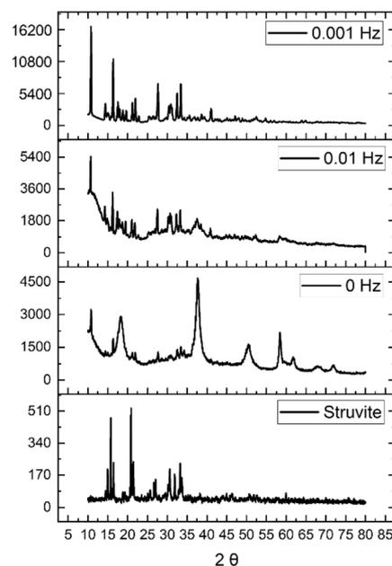
Fig. 4 X-ray diffractogram of the solid samples obtained at 53 mA and at 0.01 Hz, 0.001 Hz and 0 Hz and the struvite pattern.
