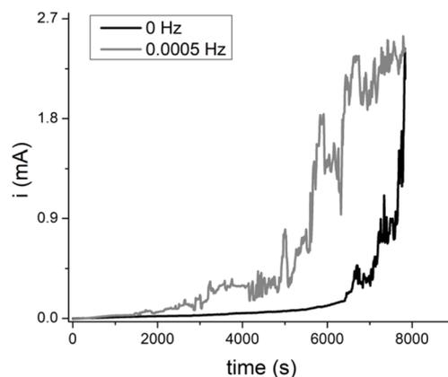
Fig. 6 Linear polarization study: working Mg electrodes operated in the electrochemical reactor at 0 Hz and 0.0005 Hz over 6 hours, in a potential window from  $-10$  to  $10 \text{ V}$  vs.  $\text{Ag|AgCl|KCl}$  at  $0.166 \text{ V s}^{-1}$  in  $0.005 \text{ mol L}^{-1}$   $\text{NaNH}_4\text{HPO}_4$ .
