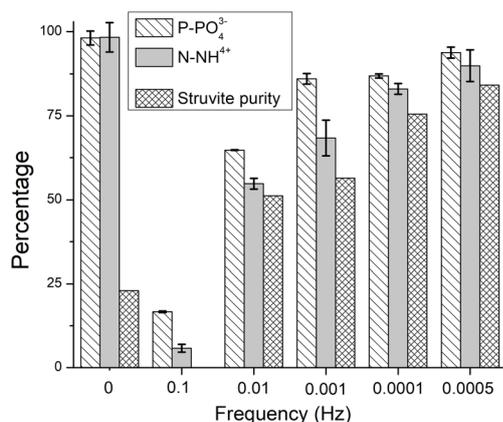
Fig. 5 Effect of frequency in the removal of  $\text{N-NH}_4^+$  and  $\text{P-PO}_4^{3-}$  and purity of struvite in the solid recovered, in  $0.005 \text{ mol L}^{-1}$  of  $\text{NaNH}_4\text{-HPO}_4$  with  $1 \text{ mg L}^{-1}$  of  $\text{NaCl}$  at  $53 \text{ mA}$ .
