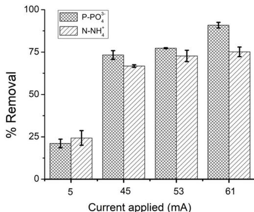
Fig. 2 Percentage removal of P-PO<sub>4</sub><sup>3-</sup> and N-NH<sub>4</sub><sup>+</sup> at different current intensities in 0.005 mol L<sup>-1</sup> of NaNH<sub>4</sub>PO<sub>4</sub>·4H<sub>2</sub>O, after 6 hours of operation in the electrochemical reactor.
