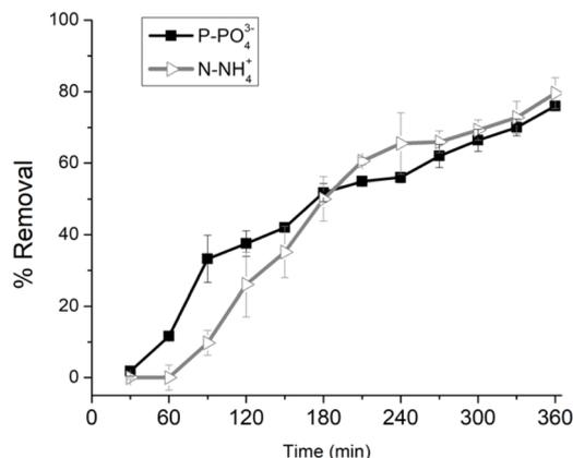
Fig. 3 Changes in the percentage of removal of  $\text{P-PO}_4^{3-}$  and  $\text{N-NH}_4^{4+}$  by an electrochemical process at 53 mA in a solution  $0.005 \text{ mol L}^{-1}$  of  $\text{NaNH}_4\text{H}_2\text{PO}_4$  over 6 h.
