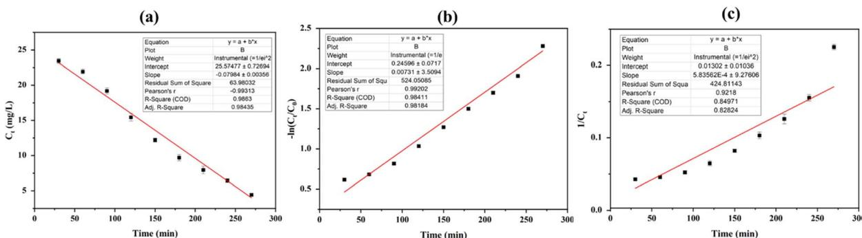
Fig. 6 Plots for RB222 degradation kinetics using  $GA@Fe_3O_4$ , (a) zero-order kinetic model, (b) first-order kinetic model, and (c) second-order kinetic model.
