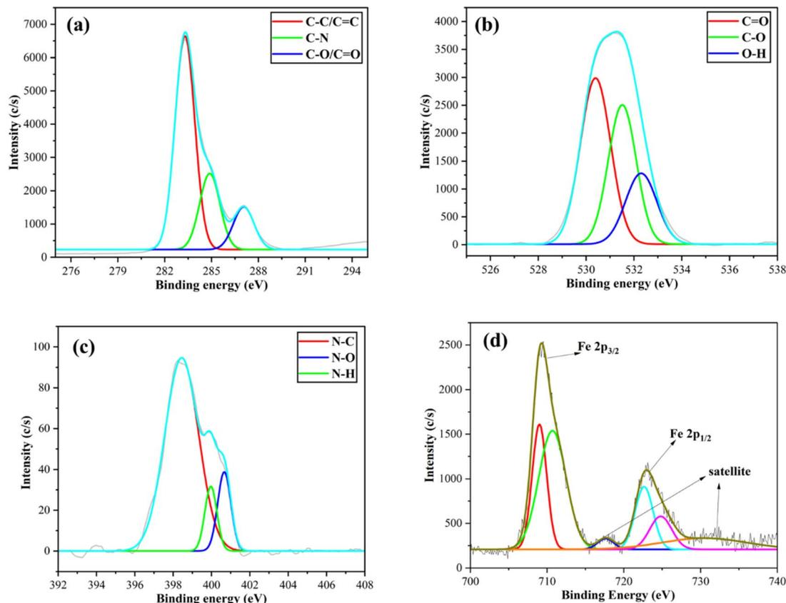
Fig. 2 XPS spectra of GA@Fe<sub>3</sub>O<sub>4</sub> with orbitals (a) C 1s, (b) O 1s, (c) N 1s, and (d) Fe 2p.
