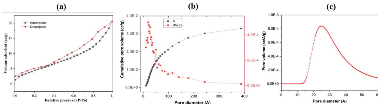
Fig. 4 (a)  $N_2$  adsorption–desorption isotherm of  $GA@Fe_3O_4$ , (b) pore size distribution of  $GA@Fe_3O_4$  determined by the BJH adsorption method, (c) pore size distribution of  $GA@Fe_3O_4$  determined by the DA method.
