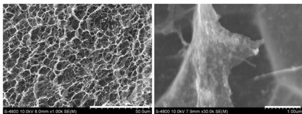
Fig. 3 SEM images of the GA@Fe<sub>3</sub>O<sub>4</sub> at two different scale bars, 50 μm (left) and 1 μm (right).
