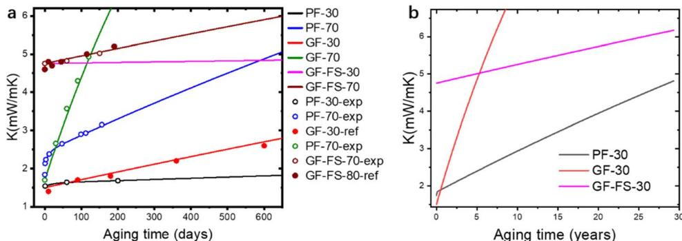
**Fig. 7** (a) Theoretical (lines) and experimental (empty dots, indicated by -exp) results and reported results from references (solid dots, indicated by -ref) of different VIP at 30 and 70°. (b) Theoretical curves of long-term (30 years) VIP aging at 30°.
