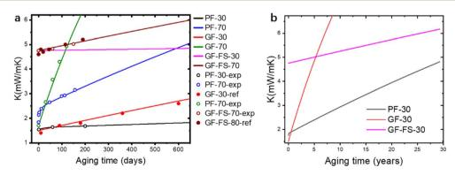
Fig. 7 (a) Theoretical (lines) and experimental (empty dots, indicated by -exp) results and reported results from references (solid dots, indicated by -ref) of different VIP at 30 and 70°. (b) Theoretical curves of long-term (30 years) VIP aging at 30°.
