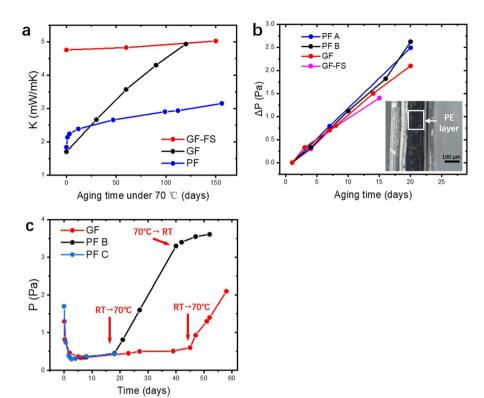
Fig. 4 (a) Thermal conductivity as the functions of aging time at 70 °C. (b) Extracted pressure increase as the function of ageing time at 70 °C. Inset: Microscopy image of the cross-section of the sealed envelope, with polyethylene layer indicated. (c) Pressure increase of three different fibers during room temperature process and 70 °C process.
