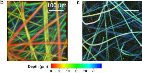
Fig. 5 (a)  $\Delta K$  as the function of  $\Delta P$  at room temperature. Inset: linear relationship of PF in the small  $\Delta P$  range. (b) Depth-coded image of PF based VIP in vacuum condition. (c) Depth-coded 3D image of GF based VIP in vacuum condition.
