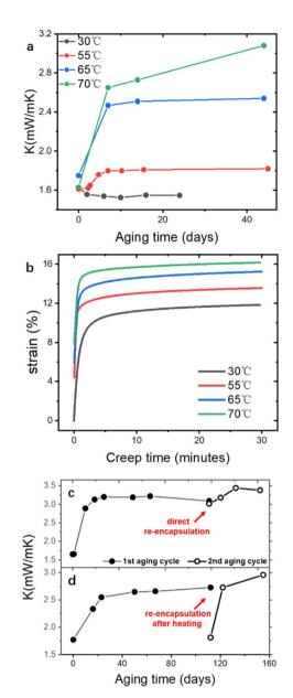
Fig. 6 (a) K aging at different temperature. (b) and (c): K aging in the first cycle and second cycle with (b) direct re-encapsulation and (c) reencapsulation after heating
