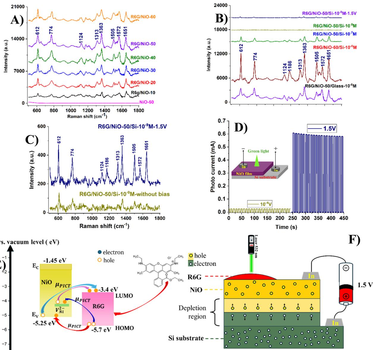
Fig. 7 Raman spectra of (A) R6G/NiO- $x$ /glass samples at  $10^{-5}$  M R6G, (B) R6G/NiO- $x$ /Si with different R6G concentration, (C) R6G/NiO- $x$ /Si at  $10^{-9}$  M R6G without bias and with 1.5 V (data in (C) are extracted from data of (B)) applied bias as Fig. 6D, (D)  $I$ - $V$  on-off characteristics  $10^{-4}$  V and 1.5 V applied bias, (E) photo induced charge transfer enhanced SERS, and (F) Raman scattering enhanced mechanism between NiO and R6G.
