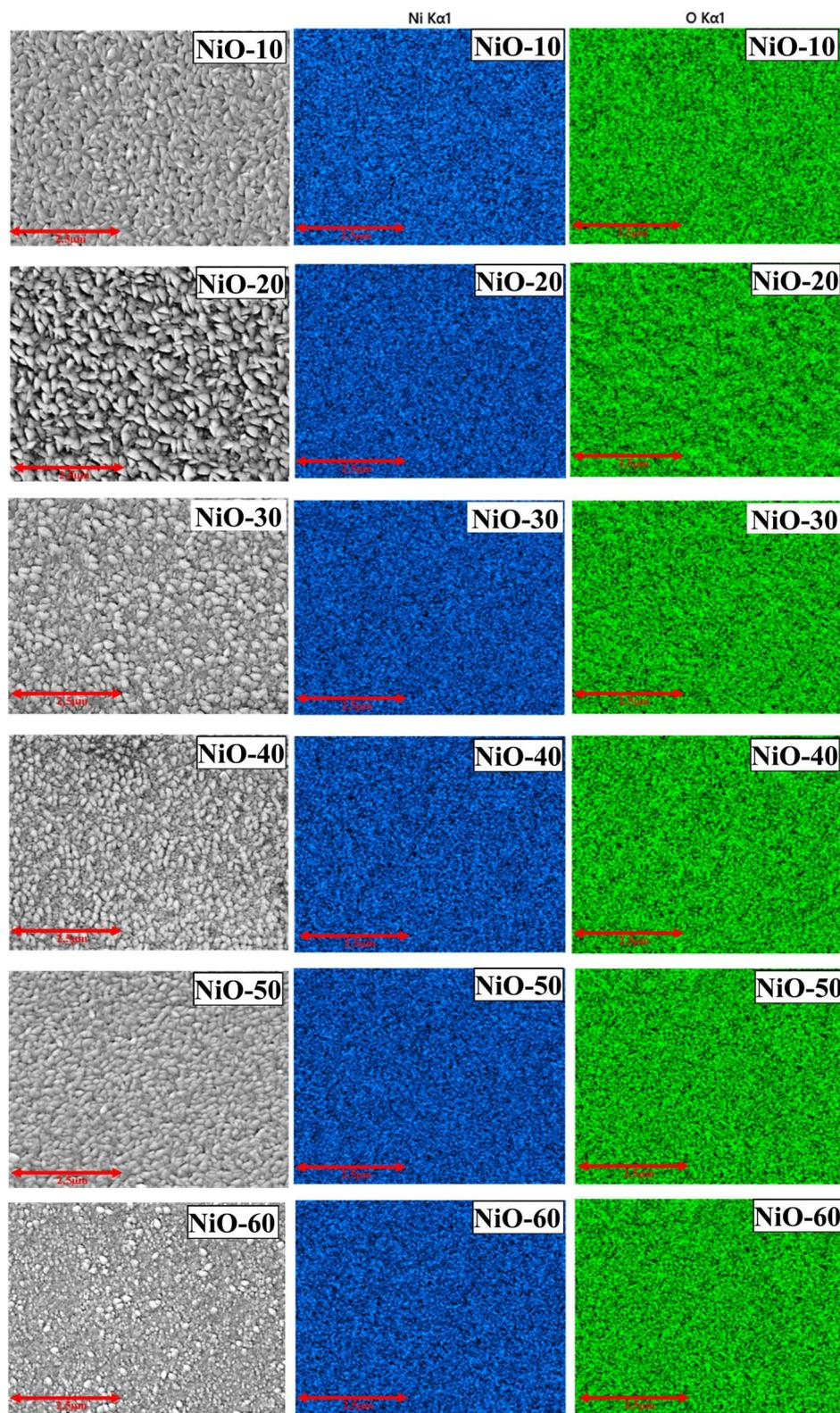
Fig. 2 EDX mapping images of NiO-x films deposited with varying O<sub>2</sub> content in the mixed sputtering gas. Columns 1, 2, and 3 show the FESEM image used for EDX scanning, the Ni elemental mapping (blue color), and the O elemental mapping (green color), respectively.
