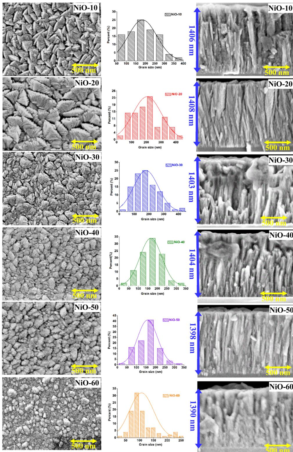
Fig. 5 FESEM images of NiO-*x* films deposited with the different O<sub>2</sub> percent in a mixed sputtering gas. Every sample is measured at a high voltage of 3.00 kV, with a working distance of around 11 mm and an 80 000 magnification.
