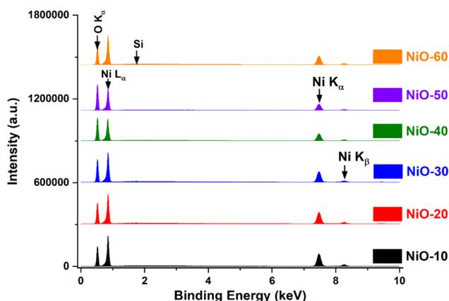
Fig. 1 EDX spectra of NiO-*x* films deposited with the different O<sub>2</sub> content in a mixed sputtering gas.
