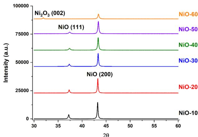
Fig. 3 XRD patterns of NiO-*x* films deposited with the different O<sub>2</sub> content in a mixed sputtering gas.
