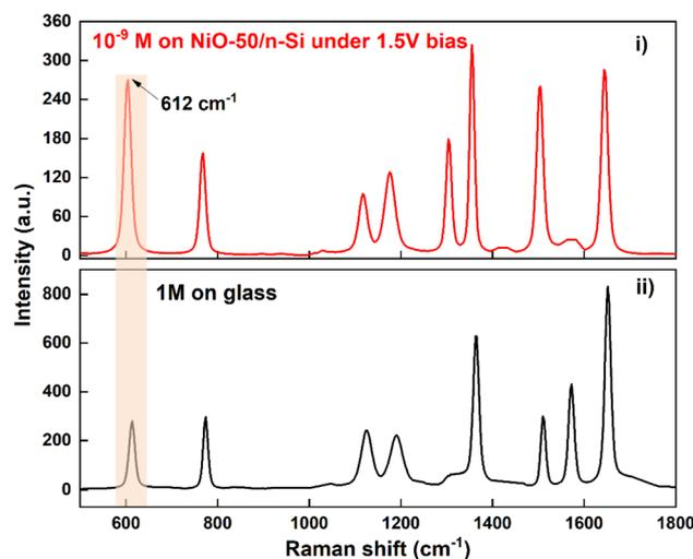
Fig. 8 The intensity of the characteristic Raman peak at 609 cm<sup>-1</sup> of the R6G molecule measured under two conditions: (i) a 10<sup>-9</sup> M R6G solution on the NiO-50/Si substrate under 1.5 V bias and (ii) a 1 M R6G solution NiO/glass substrate.
