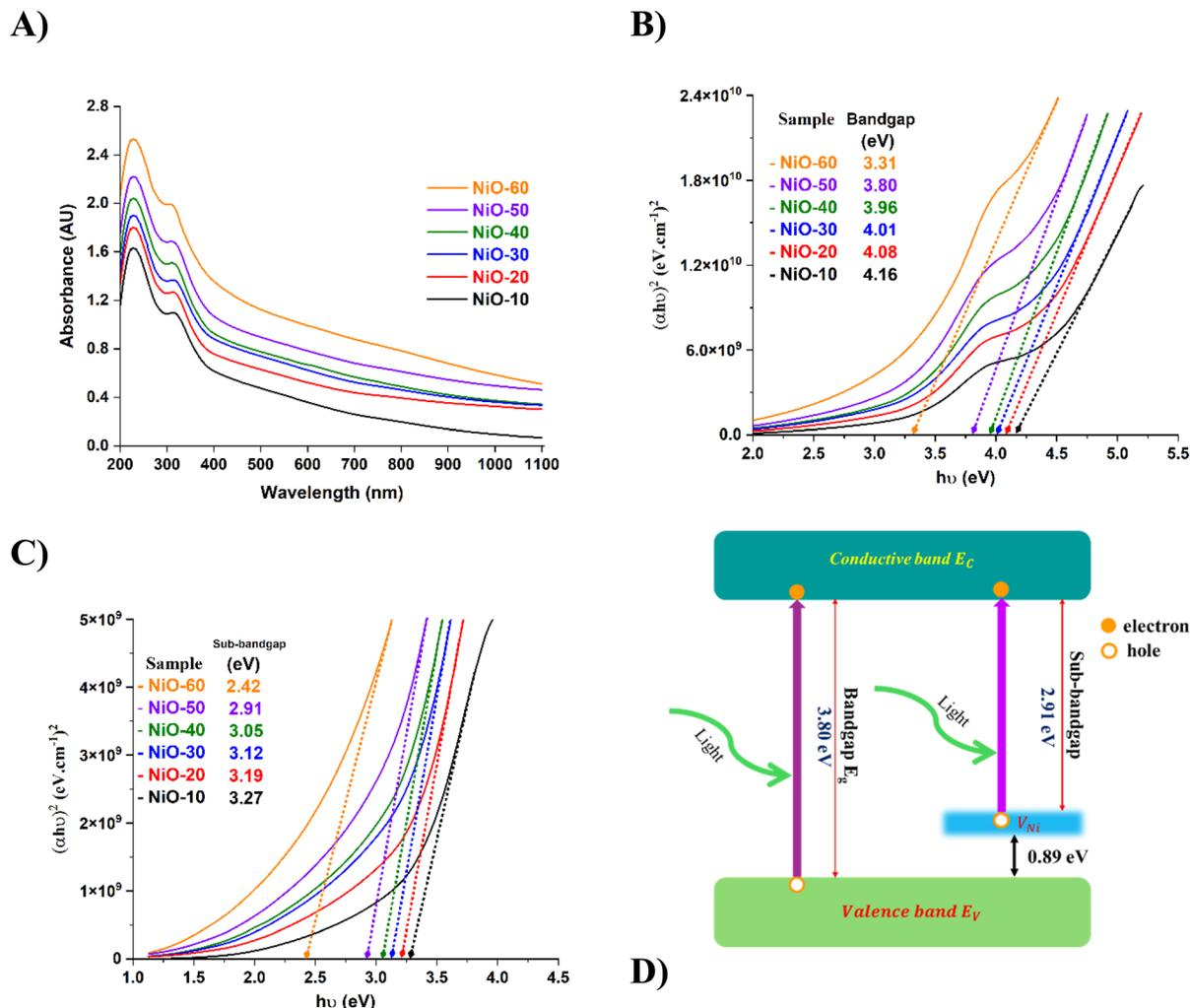
Fig. 6 (A) UV-vis spectra, (B) band gap, (C) sub-band gap, and (D) electron transition diagram of NiO-*x* films deposited with the different O<sub>2</sub> percent in a mixed sputtering gas.
