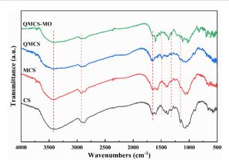
Fig. 2 FT-IR spectra of CS, MCS, QMCS, and QMCS-MO.
