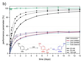
Fig. 1 Performance parameters during the degradation of (a) HMF and (b) HMB solutions of different concentrations in 1.0 M KOH. Equations of the respective Cannizzaro reaction are given to simplify color assignment. Numerical values are stated in Table S1 in the ESI.†
