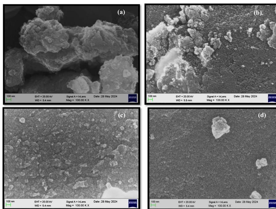
Fig. 2 FE-SEM images of IOQDs synthesized under different environments: (a) O<sub>2</sub>, (b) air, (c) N<sub>2</sub>, and (d) Ar.
