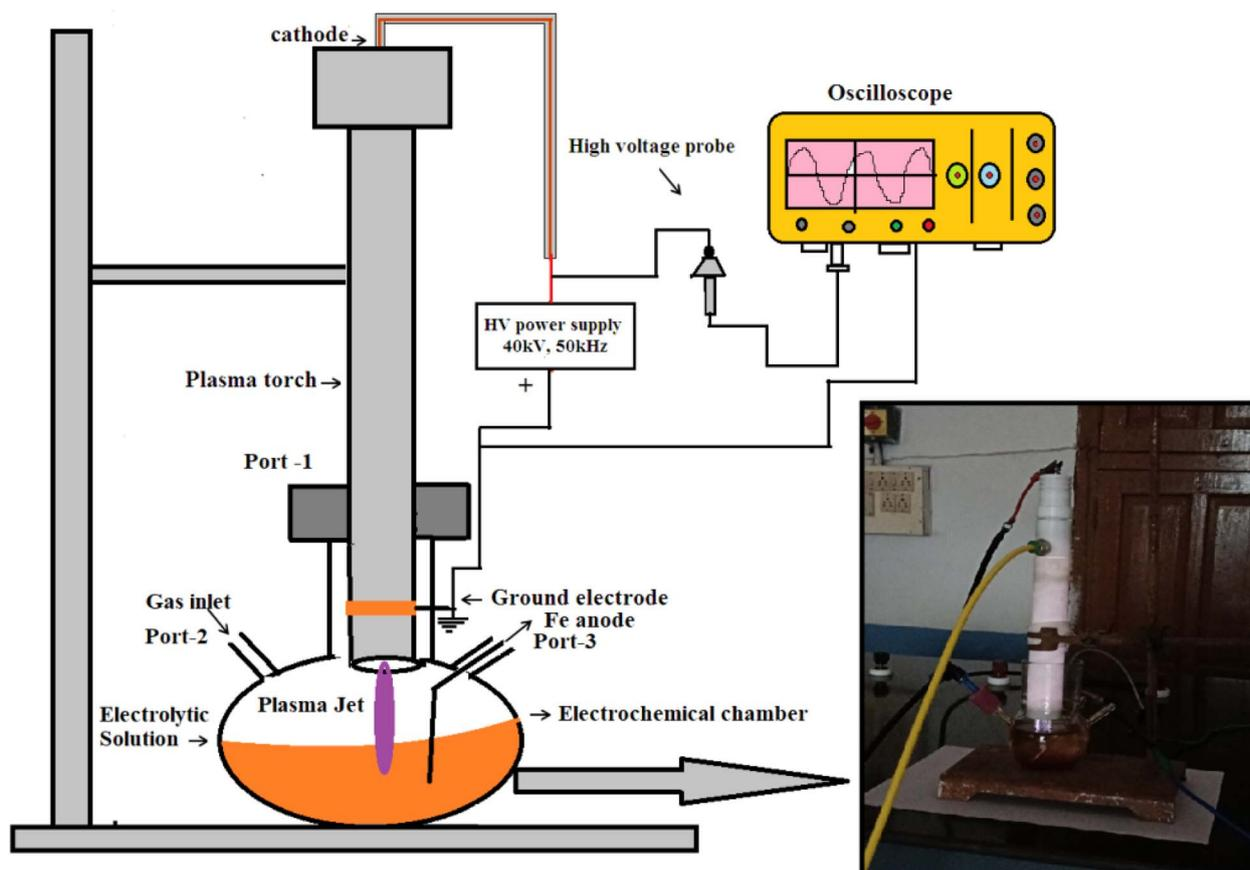
Fig. 1 Schematic diagram of the plasma electrolysis setup.
