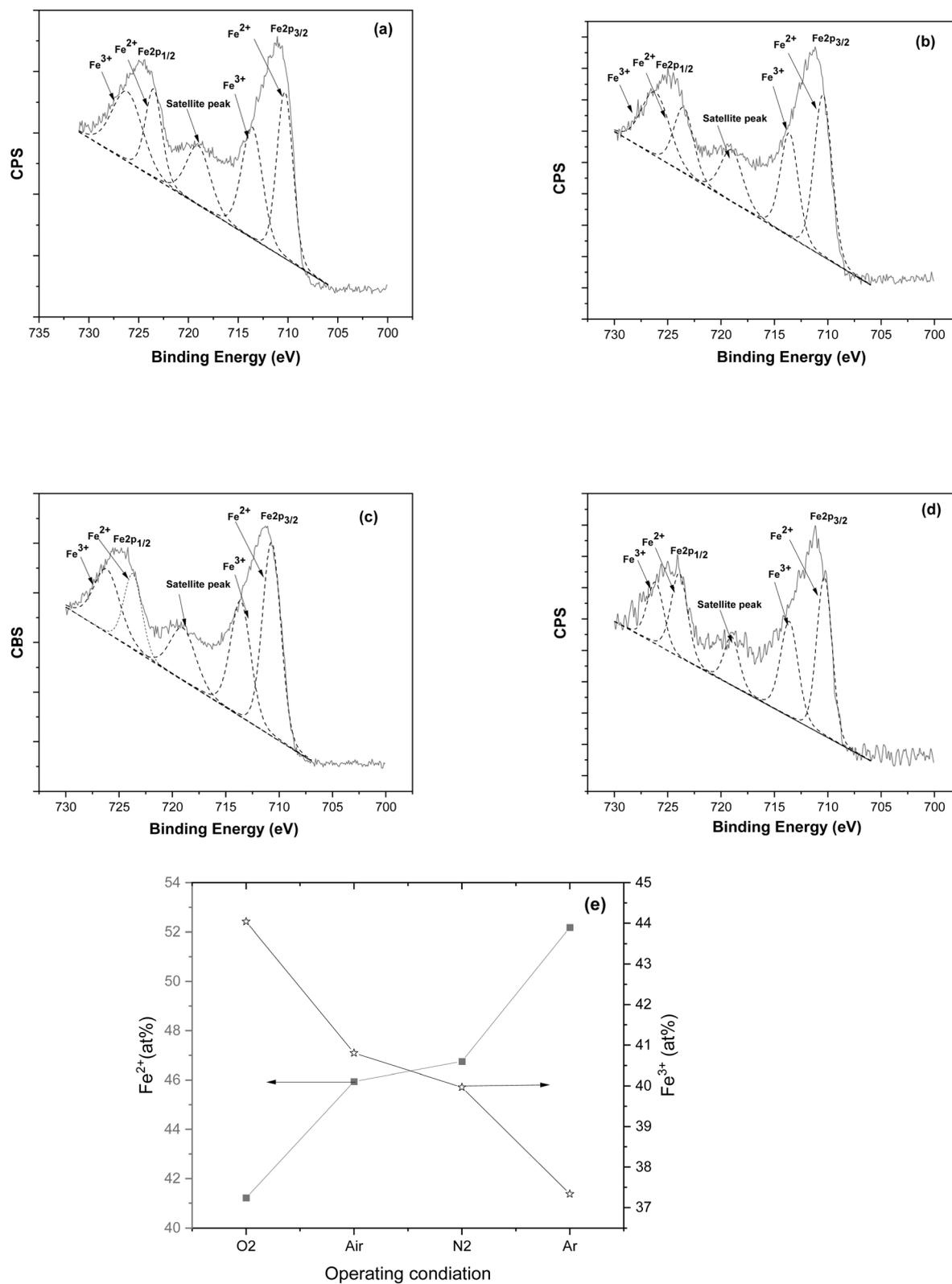
Fig. 7 High-resolution Fe 2p XPS spectra of IOQDs synthesized under different environments: (a) O<sub>2</sub>, (b) air, (c) N<sub>2</sub>, and (d) Ar. Panel (e) shows the fitted Fe 2p contributions, where peaks corresponding to Fe<sup>2+</sup> and Fe<sup>3+</sup> species are deconvoluted and labeled accordingly (Fe<sup>2+</sup> 2p<sub>3/2</sub>, Fe<sup>3+</sup> 2p<sub>3/2</sub>, Fe<sup>2+</sup> 2p<sub>1/2</sub>, Fe<sup>3+</sup> 2p<sub>1/2</sub>, and satellite peaks).
