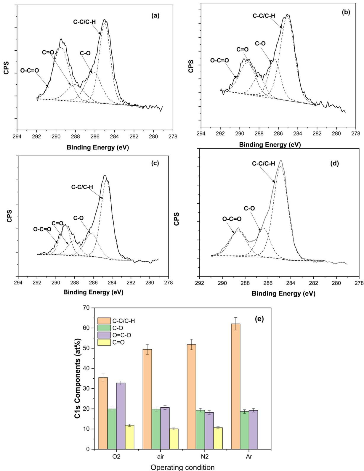
Fig. 8 High-resolution C 1s XPS spectra of IOQDs synthesized under different environments: (a) O<sub>2</sub>, (b) air, (c) N<sub>2</sub>, and (d) Ar. Panel (e) shows the deconvoluted C1s contributions, including peaks assigned to C-C/C=C (sp<sup>2</sup> carbon), C-O, C=O, and O-C=O functional groups.
