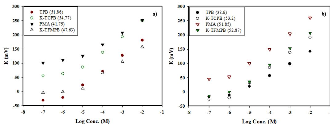
Fig. 1 (a) DON cationic exchangers (linearity ranges ( $1.0 \times 10^{-5}$  to  $1.0 \times 10^{-2}$  M) except for TPB ( $1.0 \times 10^{-6}$  to  $1.0 \times 10^{-2}$  M)), b) MEM cationic exchangers [linearity ranges ( $1.0 \times 10^{-6}$  to  $1.0 \times 10^{-2}$  M)].
