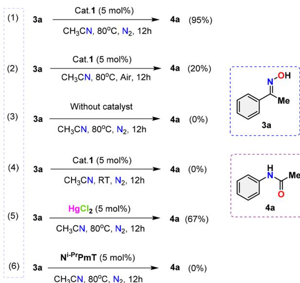
Scheme 5 Controlled experiments for investigating the mechanism.
