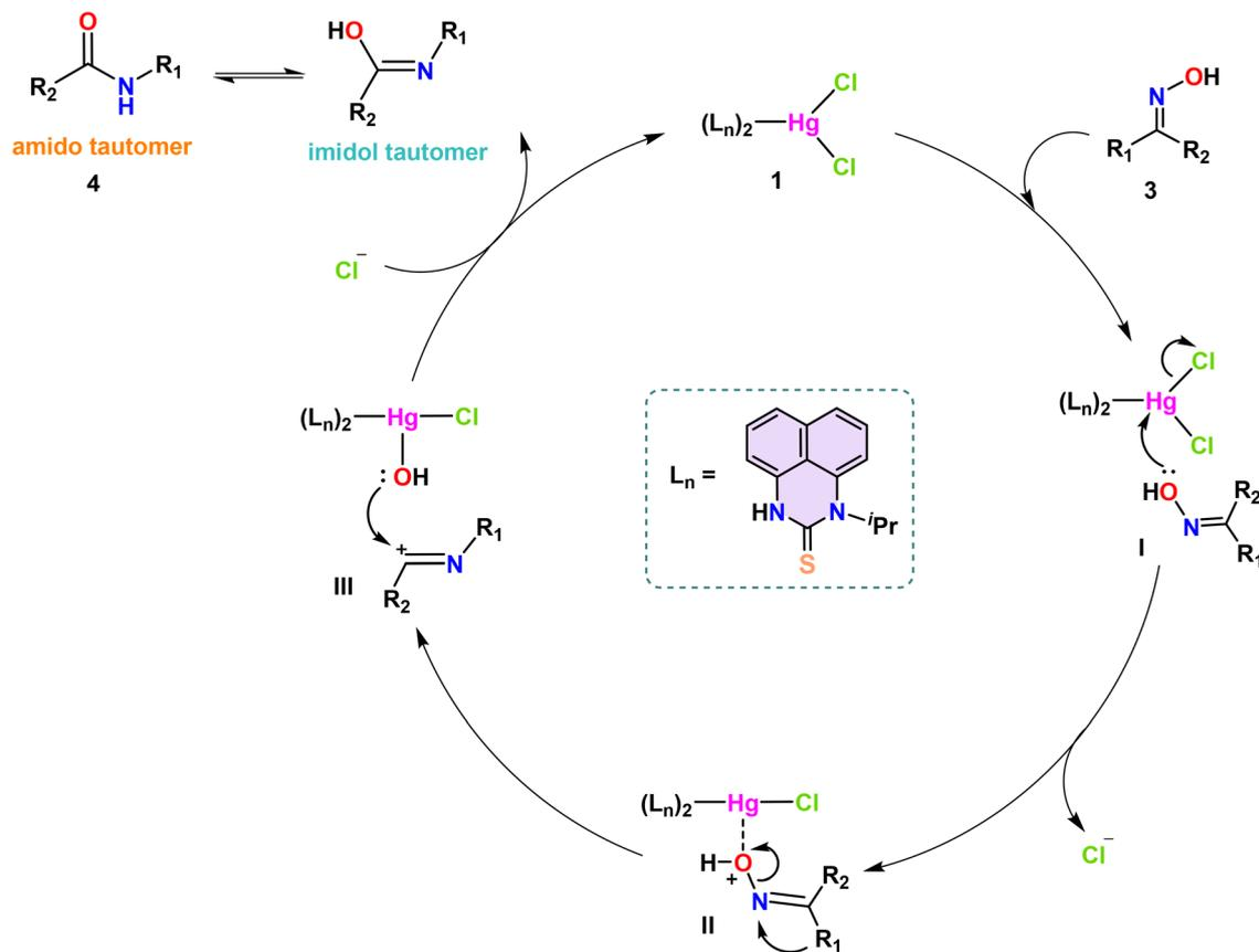
Scheme 6 Proposed mechanism for the Hg(II) complex 1-catalyzed Beckmann rearrangement of ketoximes to amides.
