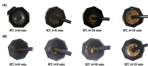
Fig. 9 Evolution of the Knoevenagel condensation reaction between (A) furfural 1a and malononitrile 2 , and (B) benzaldehyde 1h and malononitrile 2 by mechanochemistry using CS (10 wt%) as a catalyst.
