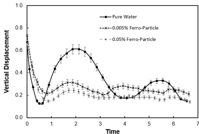
Fig. 6 Vertical displacement of rebounded droplet with dimensionless time (time is normalized by the capillary time,  $\tau_{\text{contact}} = \frac{t}{(\rho r_0^3 / \gamma)^{1/2}}$ , here  $r_0$  is the droplet radius prior to impact and  $\gamma$  is surface tension).
