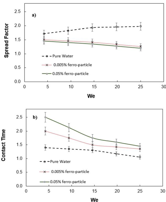
Fig. 5 Droplet spread and contact properties at mesh surface with Weber number: (a) spread factor, and (b) contact time (time is normalized by the capillary time,  $\tau_{\text{contact}} = \frac{t}{(\rho r_o^3 / \gamma)^{1/2}}$ , here  $r_o$  is the droplet radius prior to impact and  $\gamma$  is surface tension).
