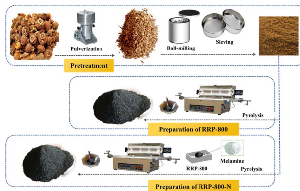
Fig. 1 Experimental flow chart for the preparation of RRP-800 and RRP-800-N.
