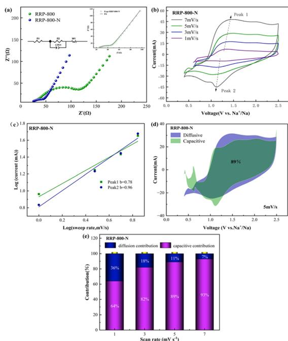
Fig. 6 (a) EIS plots. The inset is the fitting plot of RRP-800-N; (b) CV curves of RRP-800-N at different scan rates; (c) measurement of  $b$ -values of RRP-800-N; (d) contribution ratio of capacitance of RRP-800-N; (e) contribution ratio of capacitance of RRP-800-N at different scan rates.
