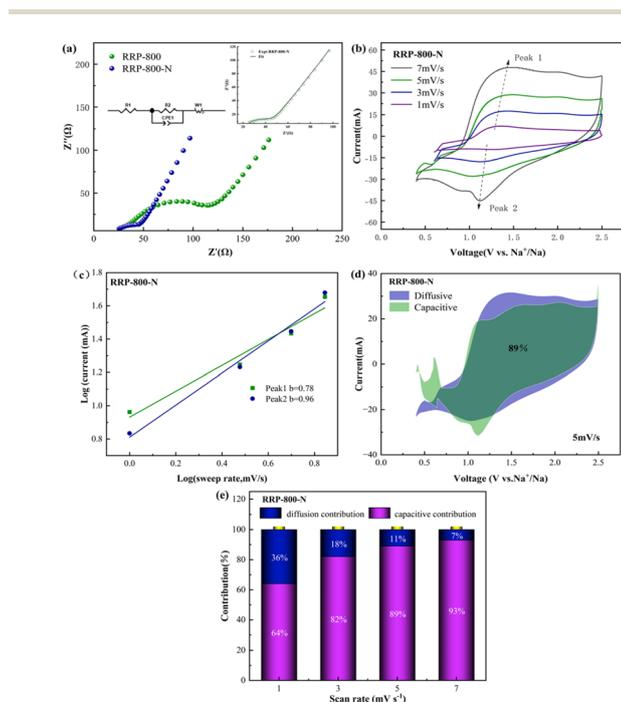
Fig. 6 (a) EIS plots. The inset is the fitting plot of RRP-800-N; (b) CV curves of RRP-800-N at different scan rates; (c) measurement of  $b$ -values of RRP-800-N; (d) contribution ratio of capacitance of RRP-800-N; (e) contribution ratio of capacitance of RRP-800-N at different scan rates.
