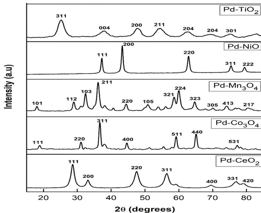
Fig. 4 p-XRD patterns of Pd-TiO<sub>2</sub>, Pd-NiO, Pd-Mn<sub>3</sub>O<sub>4</sub>, Pd-Co<sub>3</sub>O<sub>4</sub> and Pd-CeO<sub>2</sub> at wide angles.
