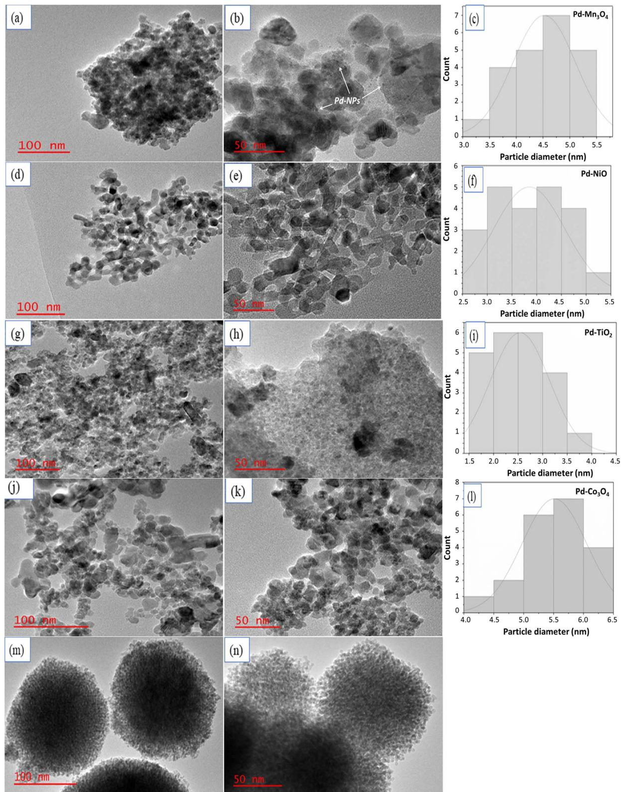
Fig. 1 TEM images of Pd-Mn<sub>3</sub>O<sub>4</sub> (a) and (b), Pd-NiO (d) and (e); Pd-TiO<sub>2</sub> (g) and (h); Pd-Co<sub>3</sub>O<sub>4</sub> (j) and (k); and Pd-CeO<sub>2</sub> (m) and (n) with their corresponding particle size distribution histograms (c), (f), (i) and (l), respectively.
