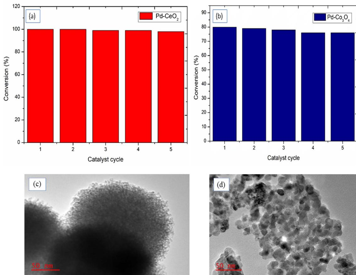
Fig. 5 Recyclability studies of (a) Pd–CeO<sub>2</sub> for Buchwald–Hartwig amination and (b) Pd–Co<sub>3</sub>O<sub>4</sub> for Sonogashira coupling; TEM images of recycled (c) Pd–CeO<sub>2</sub> and (d) Pd–Co<sub>3</sub>O<sub>4</sub>.
