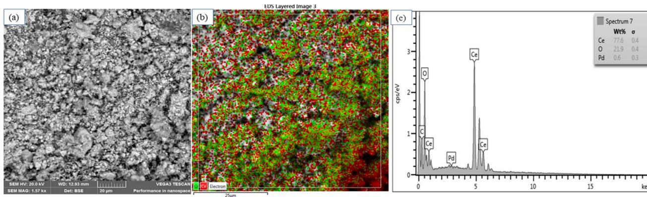
Fig. 2 (a) SEM image of Pd–CeO<sub>2</sub>; (b) elemental mapping image of Pd–CeO<sub>2</sub>; (c) SEM-EDX image of Pd–CeO<sub>2</sub>.
