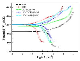
Fig. 7 Polarization curves of carbon steel in CO $_2$ -saturated 0.5 mol per L NaCl solution with 100 mg per L UiO-66-X@8-HQ (X = -H/-CH $_3$ /-NH $_2$ ) at 25 °C.
