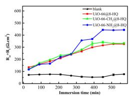
Fig. 9 Time dependence of  $R_{ct}$  +  $R_f$  for carbon steel in CO<sub>2</sub>-saturated 0.5 mol per L NaCl solution containing 100 mg per L UiO-66-X@8-HQ ( $X = -H/-CH_3/-NH_2$ ) at 25 °C.
