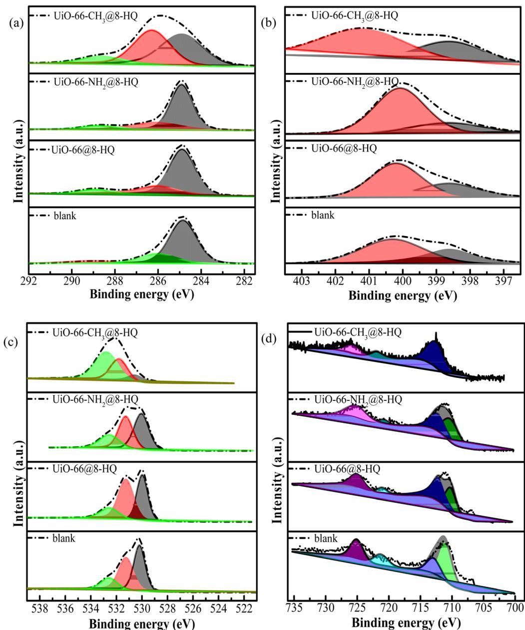
Fig. 13 High-resolution XPS spectra of carbon steel in  $\text{CO}_2$ -saturated 0.5 mol per L NaCl solution with UiO-66-X@8-HQ ( $X = -\text{H}/-\text{CH}_3/-\text{NH}_2$ ) for 24 h at 25 °C (a), C 1s, (b) N 1s, (c) O 1s and (d) Fe 2p.
