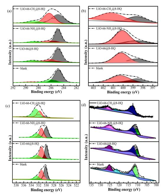
Fig. 13 High-resolution XPS spectra of carbon steel in  $CO_2$ -saturated 0.5 mol per L NaCl solution with UiO-66-X@8-HQ (X = -H/-CH<sub>3</sub>/-NH<sub>2</sub>) for 24 h at 25 °C (a), C 1s, (b) N 1s, (c) O 1s and (d) Fe 2p
