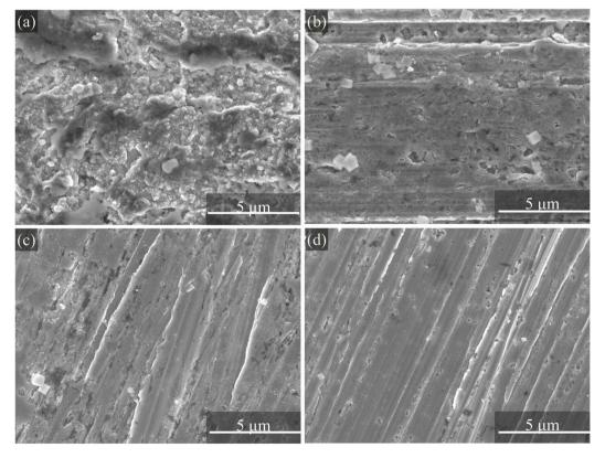
Fig. 11 SEM images of carbon steel samples immersed in CO<sub>2</sub>-saturated 0.5 mol per L NaCl solution containing 100 mg per L UiO-66-X@8-HQ ( $X = -H/-CH_3/-NH_2$ ) for 24 h at 25 °C (a) blank, (b) UiO-66@8-HQ, (c) UiO-66-CH<sub>3</sub>@8-HQ and (d) UiO-66-NH<sub>2</sub>@8-HQ.
