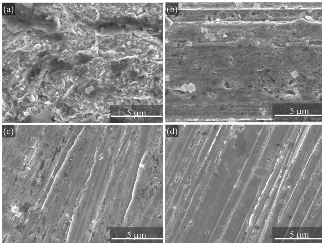
Fig. 11 SEM images of carbon steel samples immersed in CO<sub>2</sub>-saturated 0.5 mol per L NaCl solution containing 100 mg per L UiO-66-X@8-HQ (X = -H/-CH<sub>3</sub>/-NH<sub>2</sub>) for 24 h at 25 °C (a) blank, (b) UiO-66@8-HQ, (c) UiO-66-CH<sub>3</sub>@8-HQ and (d) UiO-66-NH<sub>2</sub>@8-HQ.
