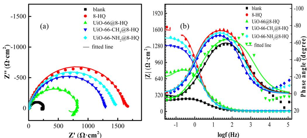
Fig. 8 (a) Nyquist and (b) Bode plots of carbon steel in  $\text{CO}_2$ -saturated 0.5 mol per L NaCl solution containing 100 mg per L UiO-66-X@8-HQ ( $X = -\text{H}/-\text{CH}_3/-\text{NH}_2$ ) at 25 °C.
