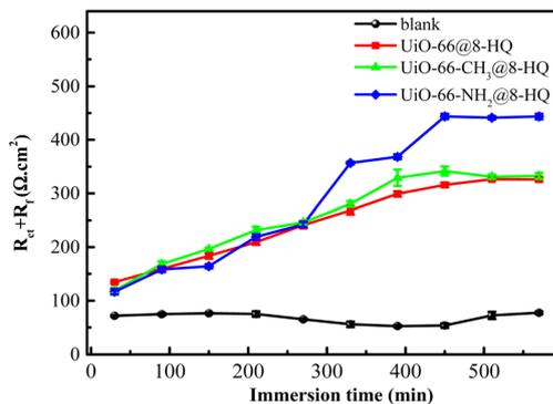
Fig. 9 Time dependence of  $R_{ct} + R_f$  for carbon steel in  $\text{CO}_2$ -saturated 0.5 mol per L NaCl solution containing 100 mg per L UiO-66-X@8-HQ ( $X = -\text{H}/-\text{CH}_3/-\text{NH}_2$ ) at 25 °C.
