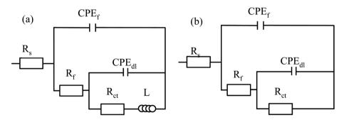
$\label{eq:Fig. 10} \textbf{ Electrochemical equivalent circuits for fitting the EIS (a) blank (b) UiO-66-X@8-HQ (X = -H/-CH_3/-NH_2). }$
