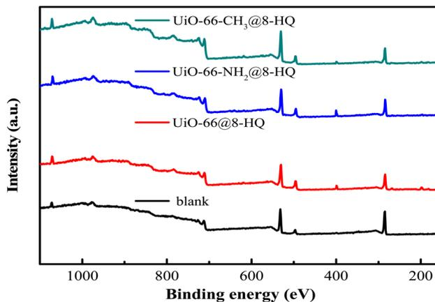
Fig. 12 Full-survey XPS spectra of carbon steel in CO<sub>2</sub>-saturated 0.5 mol per L NaCl solution containing 100 mg per L UiO-66-X@8-HQ (X = -H/-CH<sub>3</sub>/-NH<sub>2</sub>) for 24 h at 25 °C.
