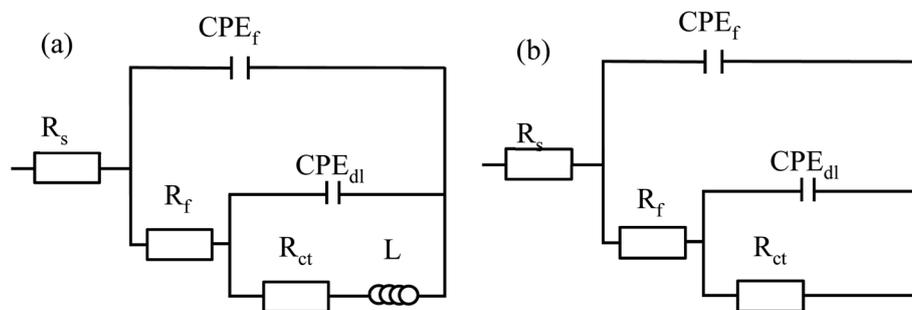
Fig. 10 Electrochemical equivalent circuits for fitting the EIS (a) blank (b) UiO-66-X@8-HQ ( $X = -\text{H}/-\text{CH}_3/-\text{NH}_2$ ).
