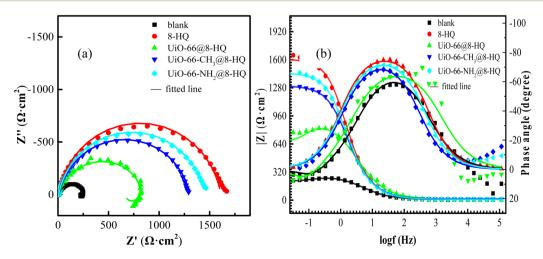
Fig. 8 (a) Nyquist and (b) Bode plots of carbon steel in  $CO_2$ -saturated 0.5 mol per L NaCl solution containing 100 mg per L UiO-66-X@8-HQ (X =  $-H/-CH_3/-NH_2$ ) at 25 °C.
