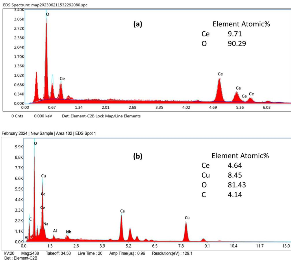
Fig. 2 EDAX spectrum of (a) nanocrystalline CeO<sub>2</sub> and (b) CeO<sub>2</sub>-CuO nanocomposite.
