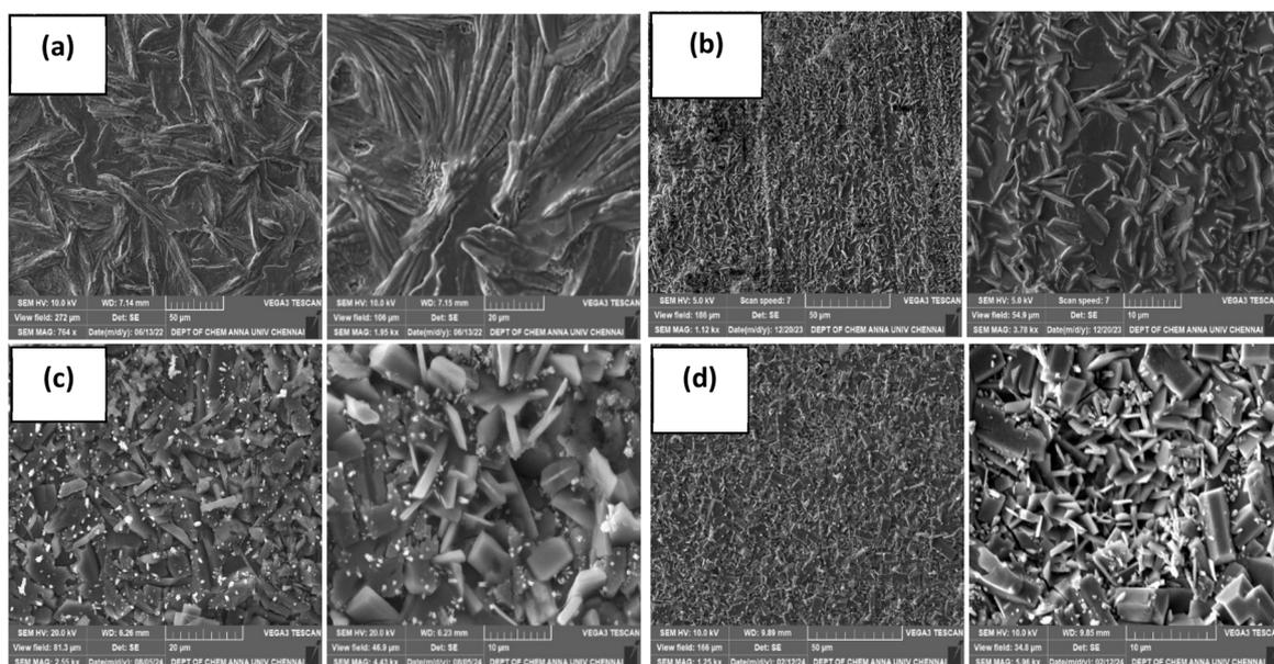
Fig. 8 Surface morphology of zinc phosphate coating formulated with different amounts of  $\text{CeO}_2$ -CuO nanocomposite. (a) ZnP; (b) ZnP-0.3COCO; (c) ZnP-0.6COCO; and (d) ZnP-0.9COCO (right side images are magnified, scale bar = 10  $\mu\text{m}$ ).
