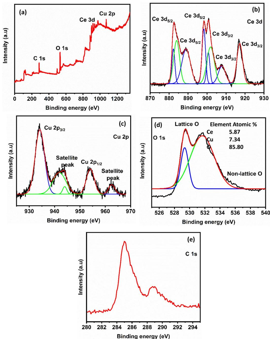
Fig. 5 (a) XPS spectrum of CeO<sub>2</sub>-CuO nanocomposite, (b) high resolution spectrum of Ce 3d, (c) high resolution spectrum of Cu 2p, (d) high resolution spectrum of O 1s and (e) high resolution spectrum of C 1s.
