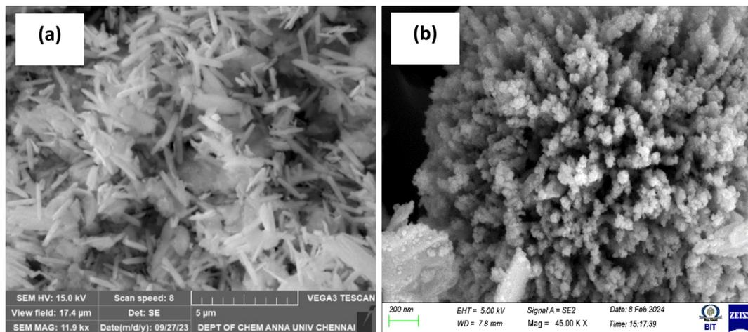
Fig. 1 SEM micrograph of (a) nanocrystalline CeO<sub>2</sub> (scale bar = 5 μm) and (b) CeO<sub>2</sub>-CuO nanocomposite (scale bar = 200 nm).
