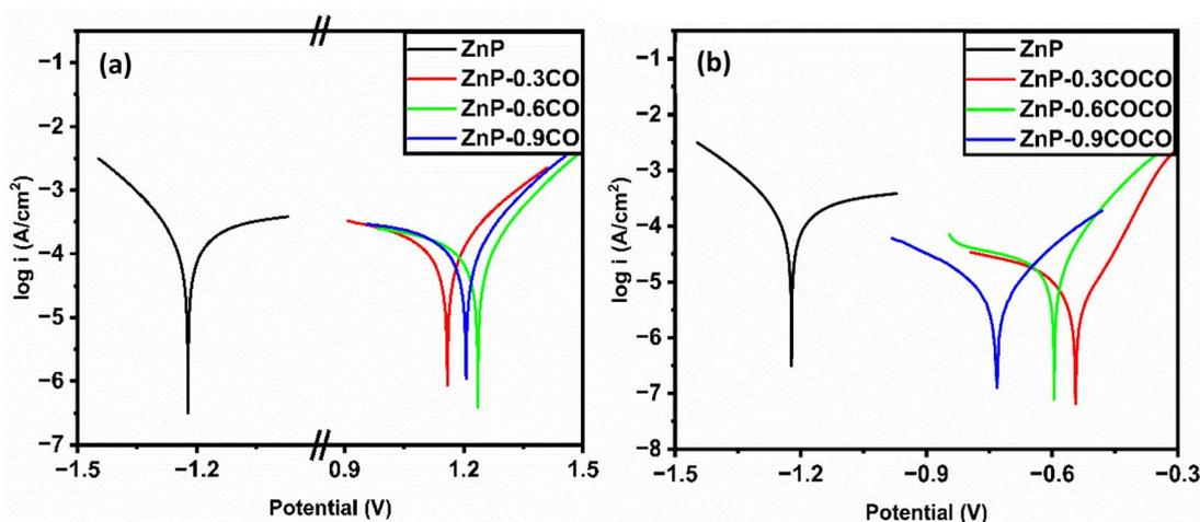
Fig. 9 Potentiodynamic polarisation curves of the uncoated and zinc phosphate coated steel substrates immersed in 3.5% NaCl. Coatings were formulated with different amounts of (a) nanocrystalline CeO<sub>2</sub> and (b) CeO<sub>2</sub>-CuO nanocomposite.
