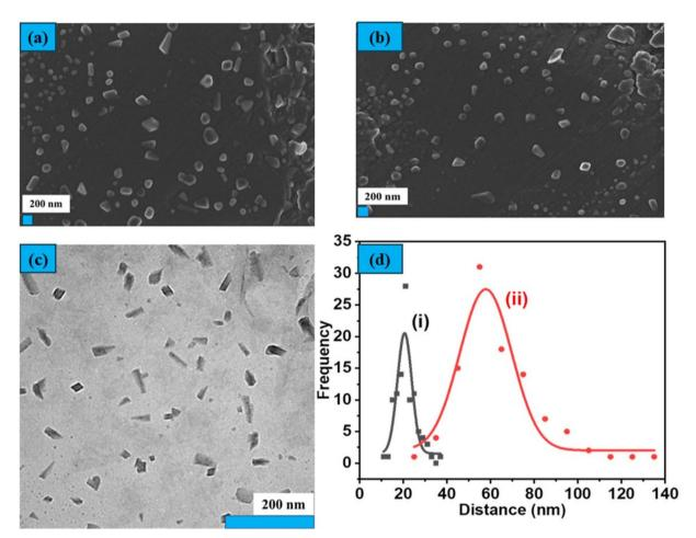
Fig. 4 SEM images of CuNRs incorporated in PEDOT:PSS for (a) 10  $\mu$ L and (b) 20  $\mu$ L, (c) TEM image of CuNRs and (d) Gaussian distribution in terms of (i) width and (ii) length.
