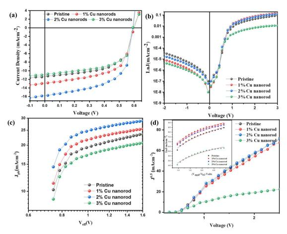
Fig. 6 (a) J-V curves of PSCs with and without CuNRs under illumination; (b) J-V characteristics of the corresponding PSCs measured under dark conditions; (c)  $J_{ph}-V_{eff}$  curves of devices incorporating different concentrations of CuNRs; and (d)  $J^{0.5}-V$  plots under dark conditions. Inset: space-charge limited current (SCLC) fitting using the Mott–Gurney law for pristine and CuNR-incorporated HTLs at varying concentrations.
