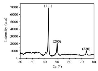
Fig. 3 X-ray diffraction pattern of synthesized CuNRs.
