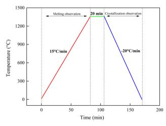
Fig. 4 Temperature control procedure of HTSOM test
