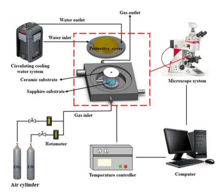
Fig. 3 Schematic diagram of HTSOM.
