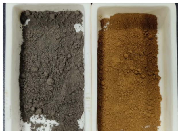
Fig. 6 Comparison of ash slag before and after ashing.
