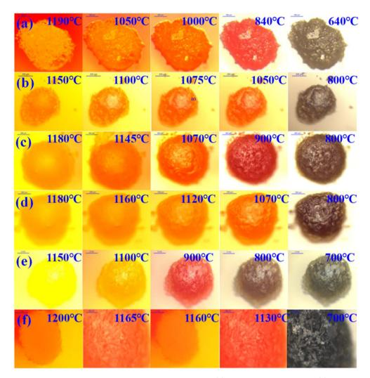
Fig. 10 In situ crystallization observation of ash slag at different positions of the RSC during the cooling process: (a) radiation screen top 25 m; (b) 25 m around spray water; (c) 20 m around spray water; (d) 15 m around spray water; (e) floating ash on water-cooled wall; (f) boiler bottom 0-1 m.
