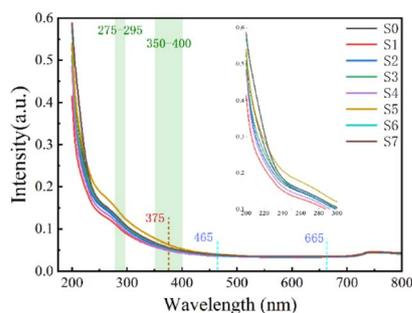
Fig. 2 UV-vis absorption spectra of water samples S0–S7. The red lines indicate the absorption coefficient ( $a$ ) values, the blue lines represent the spectral range for the ratio method ( $E_4/E_6$ ), and the green lines highlight the spectral slope ( $S_R$ ) values.
