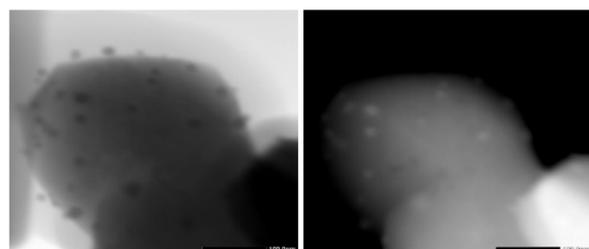
Fig. 8 Bright field-dark field images of Ag/La-ZnO Nanoparticles.
