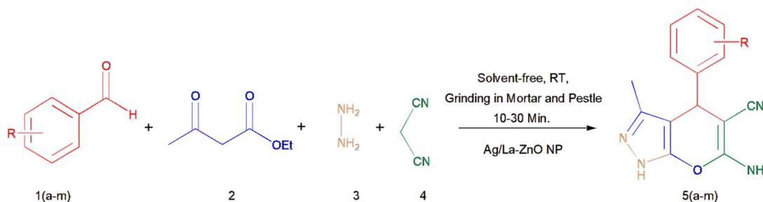
Scheme 1 Schematic representation of the solvent-free, four-component synthesis of 4*H*-pyrano[2,3-*c*]pyrazoles using aryl aldehydes, ethyl acetoacetate, malononitrile, and hydrazine hydrate *via* grinding in a mortar and pestle using the Ag/La-ZnO nanocatalyst.
