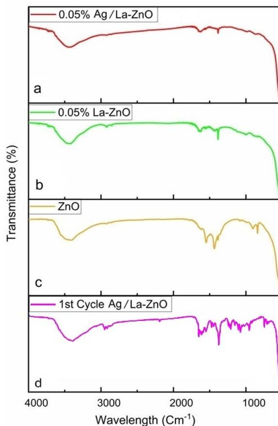
Fig. 2 FTIR spectra of undoped ZnO, La-ZnO, and  $\text{Ag/La-ZnO}$  and 1<sup>st</sup> cycle  $\text{Ag/La-ZnO}$  nanocatalysts.
