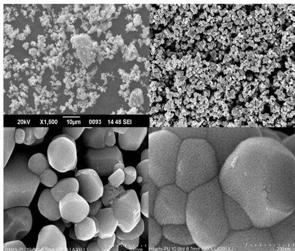
Fig. 4 SEM analysis of 0.05% Ag/La-ZnO nanoparticles.
