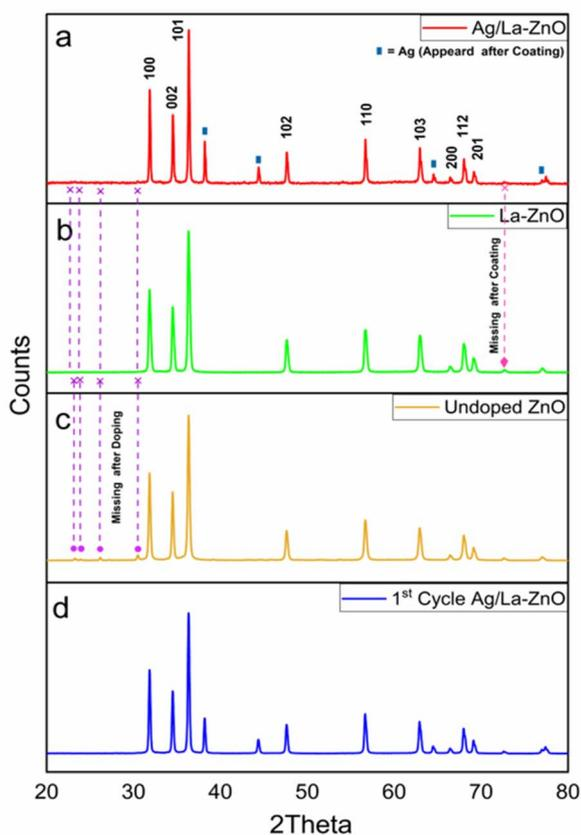
Fig. 3 The XRD pattern of (a) Ag/La-ZnO, (b) La-ZnO, (c) undoped ZnO, (d) 1<sup>st</sup> cycle Ag/La-ZnO nanocatalyst.
